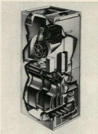
**Curved heat exchanger** eliminates creaking noises and metal fatigue problems caused by expansion of hot metal. Duracove units are designed for add-on air conditioning. From 55,000 to 220,000 BTU. Lennox, Marshalltown, Iowa. (For details check No. 27 on p. 174)
