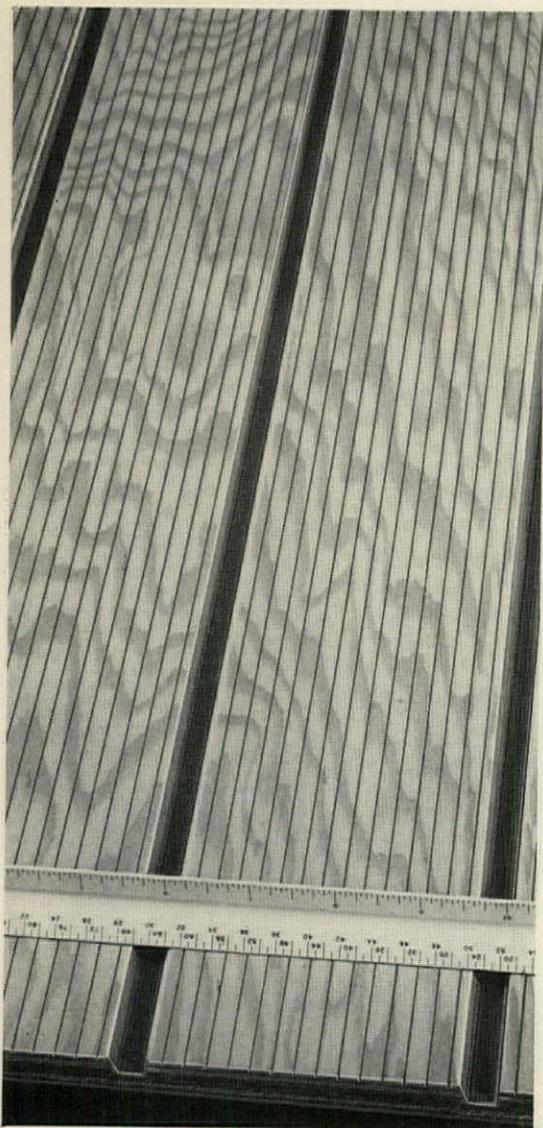
NO-CHECK pattern effectively relieves veneer surface stresses which cause checking and gives wood a rich textured appearance. NO-CHECK striations 1/32 inch wide by .080-inch deep on 1/4-inch centers run long way of panel. Shown here is T1-11 panel also available as plain NO-CHECK Panels.
