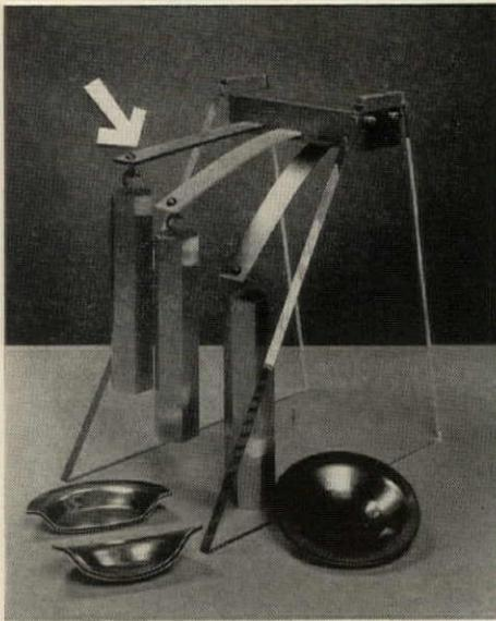
**STRENGTH TEST** shows stiffness of new laminate (arrow) vs. reinforced plastic and steel.
