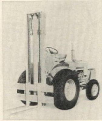
**Heavy duty forklift** is self-propelled, comes with lift heights ranging from 10½' to 21½'. High flotation tires and improved underaxle and undermast clearance help machine withstand extreme loads. International Harvester, Chicago.
