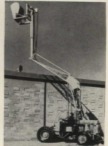
**High-lift loader** is one of ten models with reach heights up to 40' and capacities of 2,500 to 6,000 lbs. Accessories include concrete hoppers, hod buggies, buckets and workman's platforms. Lull Engineering, St. Paul, Minn. Circle 76 on Reader Service card
