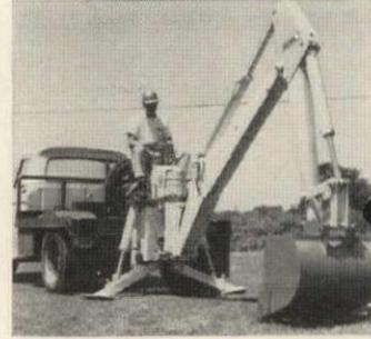
**Backhoe** is mounted on 1½-ton truck for speed and mobility. Model 180 Truck Hoe uses hydraulics to move itself off and on the truck bed. It has a 16½' reach, can dig to a 13½' depth. Seven different buckets are offered. Henry Mfg., Topeka, Kans.
