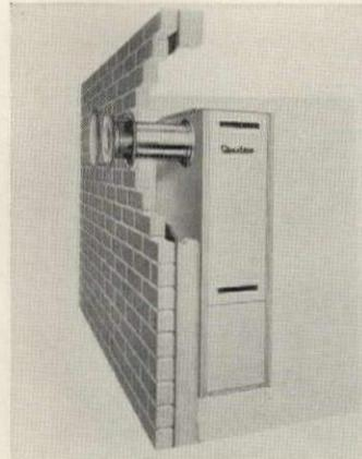
**Chimneyless gas furnace** has concentric through-wall flue to take in fresh air and exhaust combustion air. Saf-T-Sealed unit has 55,000 btu heating capacity, can also be fitted with a two-ton cooling system. Peerless Div., Louisville, Ky.
