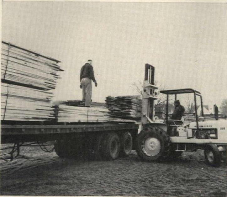
**High-lift forklift** comes with a 21' mast that has 2,500 lb. capacity at full height, 5,000 lb. capacity at 14' height. Also available: interchangeable hydraulic bucket, mortar hopper, blade and swing boom. John Deere, Moline, Ill. (Circle 74 on Reader Service card)
