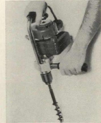
**Cordless drill** is powered by compact gasoline engine. Drill-gine has ¾ hp engine and comes in two models: ⅜"-capacity chuck with 1,360 rpm spindle speed or ½"-capacity chuck with 620 rpm speed. Orion Mfg., La Mirada, Calif.
