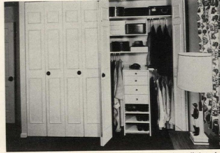
**Bi-fold closet doors** slide in a top track that can be nailed to the ceiling. New hardware design lets floor plates support doors' entire weight. Doors are made of  $\frac{3}{4}$ ", three-ply particle board. Paniflex Door, New York City. (Circle 56 on Reader Service card)
