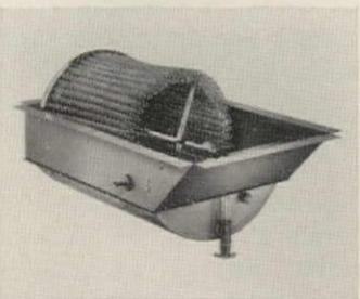
**Evaporative humidifier** fits in supply-air ducts, converts up to 22 gals. of water per day into vapor. It can be used with furnace capacities of up to 125,000 btu. Mesh element is self-cleaning, and refill is automatic. Walton Laboratories, Irvington, N.J.
