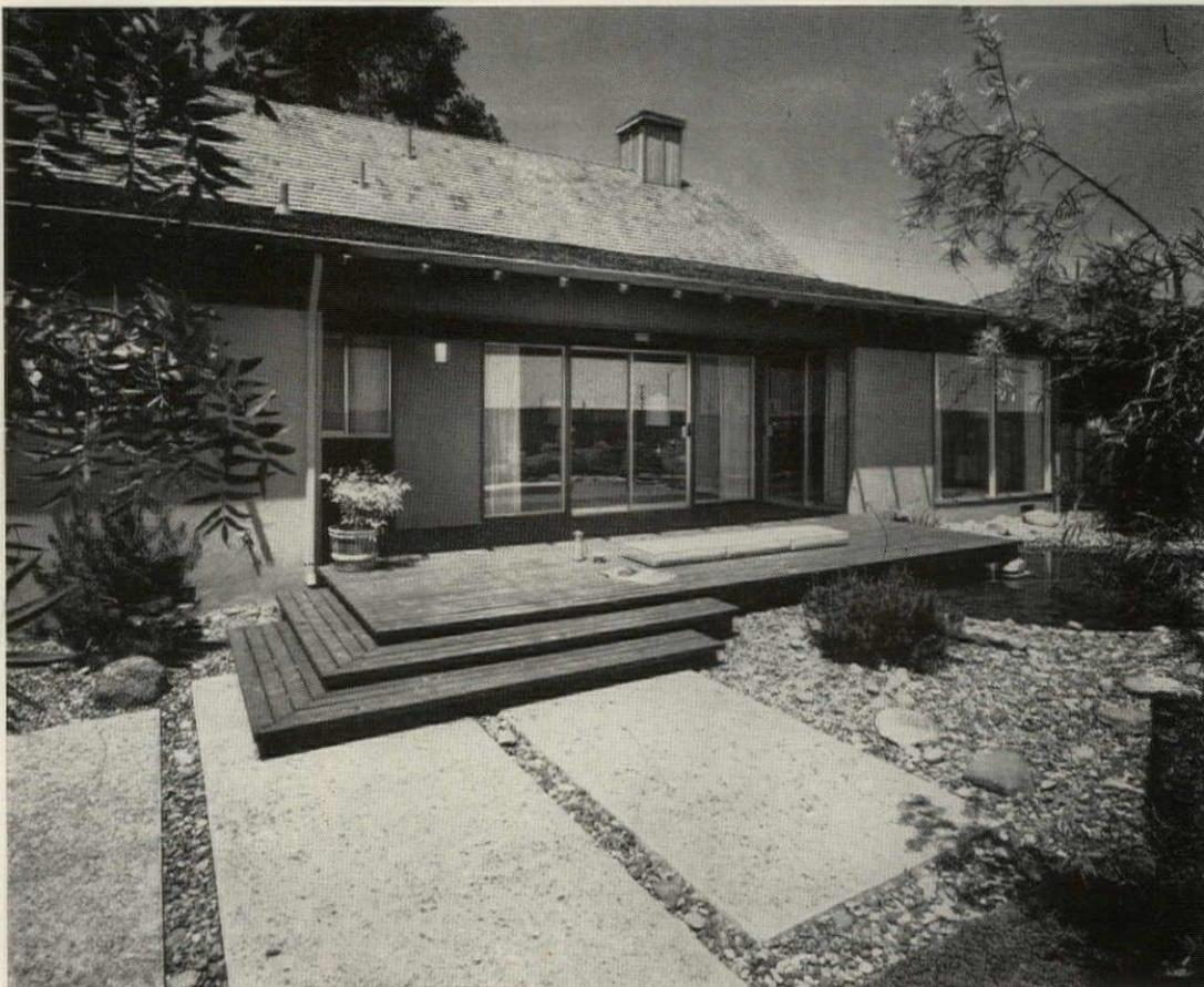
**REAR DECK** is made of redwood planks. Stone-and-cement terrace is easy to maintain.
