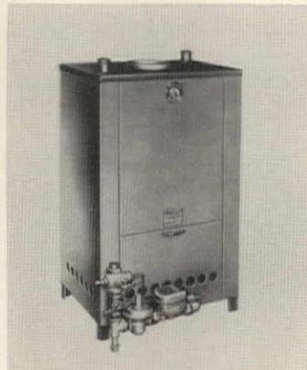
**Swimming pool heater**, fueled by gas, has 460,000 btu input, can raise the temperature of a 37,000-gal. pool 25° in 24 hours. It also maintains pool temperature automatically. Ruud heater operates on all gases, including LP. Rheem, Chicago.
