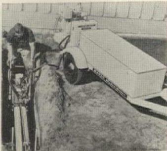
**Hydraulic borer** has its own hydraulic system, power source and mobile carrier. Power pack has 9 hp engine to drive pump. Borer has hydraulic motor with instant forward-reverse. Carriage can handle 10' drill stems. Davis Mfg., Wichita, Kans.
