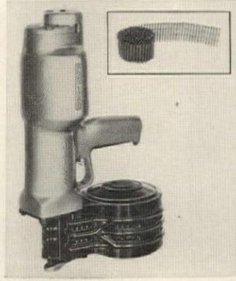
**Canister nailer** drives full-head, standard 6d or 8d common, box or sinker nails. Nails are packaged in coils of up to 300. Model N2 Common Nailer has touch-trip, semi-automatic or fully automatic control. Bostitch Inc., E. Greenwich, R.I.
