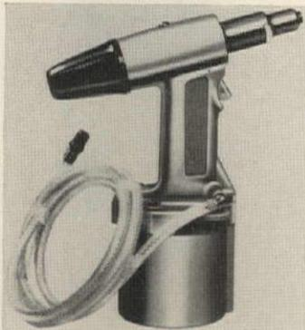
**Pop riveter** of air-hydraulic type handles rivets in sizes of 3/8" up to 1/2" in diameter. Model PRG 540 weighs only 4½ lbs. It requires an 80 psi air supply to activate the self-contained hydraulic system. United Shoe Machinery, Shelton, Conn. Circle 77 on Reader Service card
