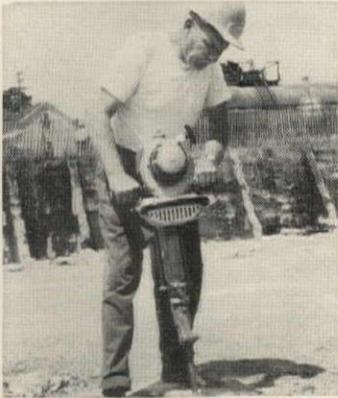
**Utility breaker** can be used to remove old concrete floors or stone or to loosen compacted soil, clay or gravel. In addition, model UB-25 can be used for tamping, pipe laying and post setting. Wacker Corp., Hartford, Wis.
