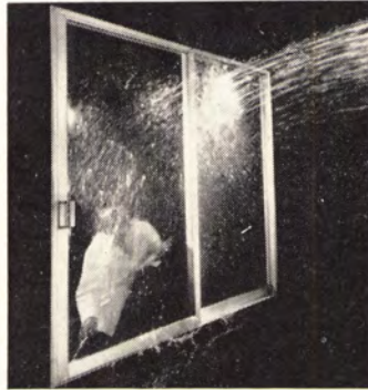
Sliding glass door is said to block water infiltration with a nonsiphoning sill that works on a pressure equalization principle. Doors come in light bronze, medium bronze and black finishes. Threshold is weatherstripped. Kawneer Co., Niles, Mich. (Circle 312 on Reader Service card)
