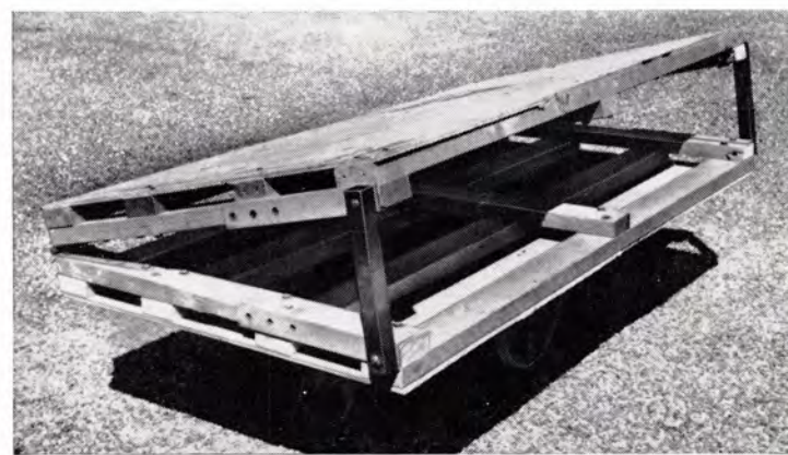
ROOF-LEVEL PLATFORM that adjusts to pitch holds plywood stack close to job. Another idea: sharpened hammer claws help workmen position panels.
