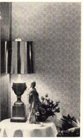
Plastic - finished hardboard in Chantilly design comes in beige, green, gold and rose. The 4'-wide panels are said to be suitable for all interior surfaces. They are ½" thick, installed with wallboard adhesive. Marlite Paneling, Dover, Ohio.
