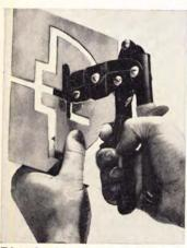
Plastic laminate shear cuts melamine counter materials in scrolls, circles, angles and straight cuts. Its patented alloy blades don't chip or mar decorative surfaces. The Klenk Plastic Laminate shear retails for \$12.50. Karl Klenk Inc., Wilmington.
