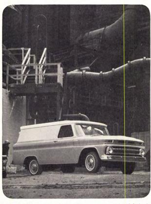
PANELS You have a choice of ½-ton panel with 7½-ft. body or an extra-long 1-ton model with 10½-ft. body. Both feature smooth laminated wood floors with full-length steel skid strips to help move cargo easily in or out through large double rear doors.
