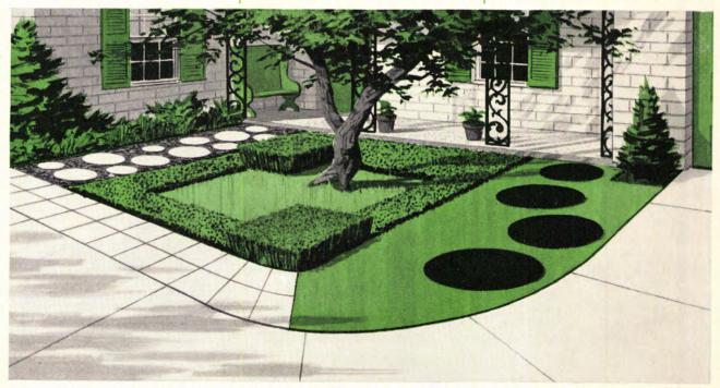
"Turning a yard into a selling feature is simple with concrete." In this design, Mr. Klopp shows a walk of precast concrete rounds set in exposed aggregate concrete made with black Japanese pebbles. This contrasts beautifully with a driveway landing strip of
