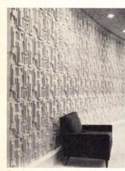
**Sculptured panels** are precast and come in four finishes: natural gray, smooth and etched white and buff. Wall-facing units weigh 35 lbs. and are 15<sup>3</sup>4" square with a basic thickness of 1½". Nitterhouse Concrete Prods., Chambersburg, Pa.
