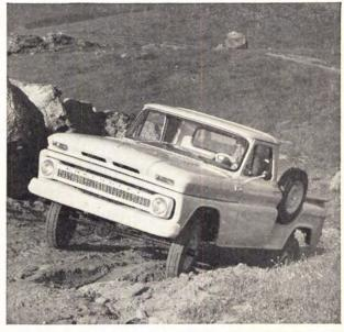
4-WHEEL-DRIVES Available in ½- and ¾-ton chassis in a whole range of models—pickups, Carryalls, panels, chassiscabs. Give versatile go-anywhere traction for tough off-road assignments. Include 2-speed transfer case,
