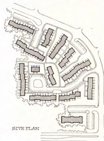
SITE PLAN groups townhouse apartments in straight rows for maximum use of sloping land.
