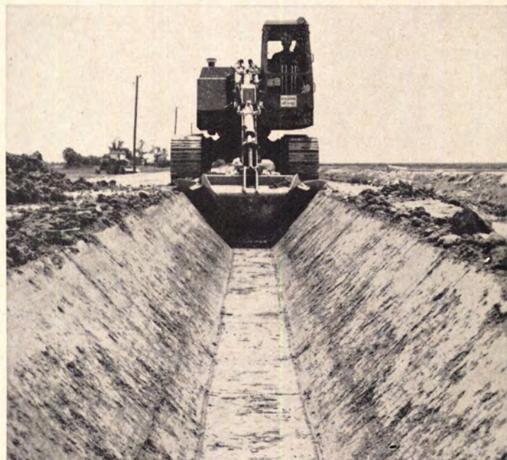
Drainage ditch excavator has V-shaped bucket that excavates trenches with a 12" flat bottom and a maximum 71" width. It digs smooth, finished ditches in a single pass without clean-up or hand work. American Poclain, Rahway, N.J. (Circle 224 on Reader Service card)
