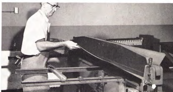
POWER BREAK is one of three 8' machines to permit prefabricating of standard 8'-long duct.
