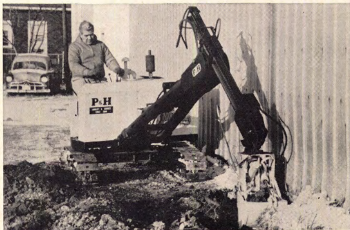
Small excavator has 2-cu.-ft. all-position bucket, a low silhouette and only 3.7 psi ground pressure which permits it to be used to dig beside existing buildings. It can dig to a depth of 11 ft. Harnischfeger, Milwaukee. (Circle 227 on Reader Service card)
