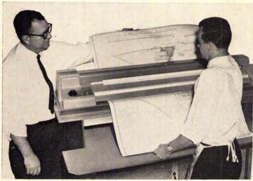
Whiteprinter, called Diazo-Jet, reproduces plans, office forms, job sheets and other office papers in less time and at reduced expense, according to the manufacturer. Price: \$595. Seven models available. Rotolite, Stirling, N.J. (Circle 251 on Reader Service Card)
