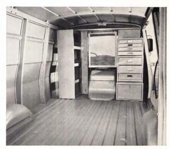
Route delivery and service installation. Plenty of space for large items, convenient bins and drawers for parts and tools.
