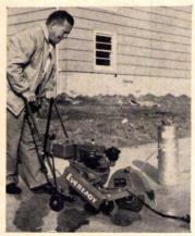
Portable concrete saw weighs 102 lbs, and can be operated by one man. Models, with 3 hp and 5 hp, can saw contraction joints in basement floors and in concrete driveways and sidewalks. A 10" diamond blade is optional. Eveready, Kansas City, Mo. Circle 241 on Reader Service card
