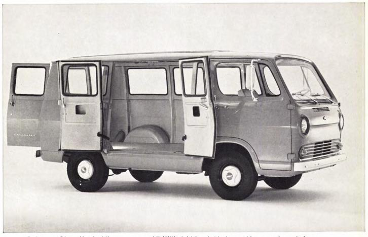
Order your Chevy-Van just the way you want it. With right-hand side doors, side or rear door windows—or 10 big windows for the 211-cu.-ft. cargo area. Order a 120- or 140-hp 6-cylinder engine up front.
