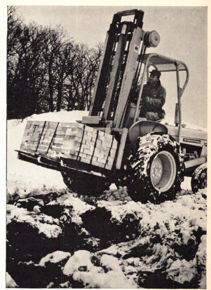
Excellent traction and flotation—key to any rough ground operation. Big, broad pneumatic tires. Generous under-axle and under-mast clearances.
