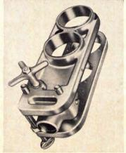
Combination jig for locksets may be used for 23/8", 23/4" or 5" backset installation. Jig is adjustable for door thicknesses from 1 5/16" to 21/4". Either hand brace or power tools can be used with the jig. Kwikset, Anaheim, Calif.
