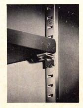
easy installation. Standards mount flush or on the surface, in minutes, with drive screw nails or staples. The 255 steel standards are available in nickel- or zinc-plated finishes, in lengths from 12" to 144". The 255-AL aluminum standards with natural aluminum or bronze vinyl finish come in 18" to 144" lengths. Supports are finished in zinc or bronze. Ask your K-V representative or send for our complete catalog.
