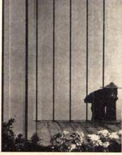
Board-and-batten siding is offered in 4'-wide panels with battens applied. Graded wood particles bonded together with synthetic resins give Par-Tex a uniform surface. Panels are 8', 9', 10' or 12' long. Forrest Inds., Portland Ore.
