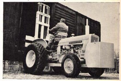
Twin hydraulic circuits let you operate tilt and hoist controls at the same time with no lag or hydraulic starvation. Side-shifter (3" right or left) is optional.
