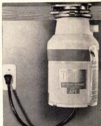
Disposer , designed for apartment installation, has factory-installed electrical cord. A self-service wrench with instructions is attached to the unit. Disposer has a three-year parts and a one-year labor warranty. In-Sink-Erator, Racine, Wis. Circle 202 on Reader Service card
