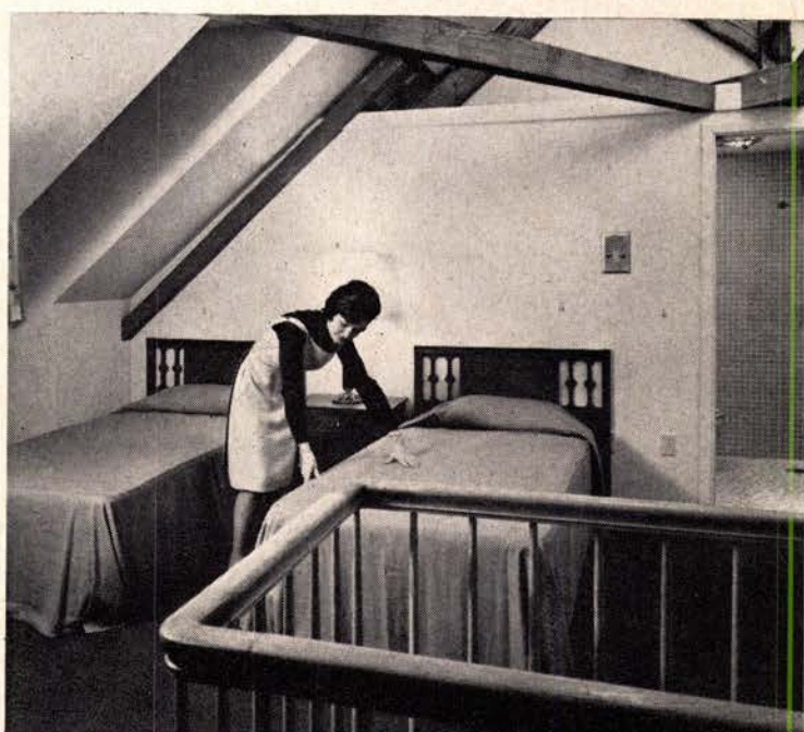
Walls and ceiling were insulated and plastered, and the original cypress beams were left exposed for effect.
