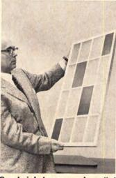
Sandwich-type panels, called Danalite, are made of glass-fiber reinforced acrylic modified polyester. The panels come in thicknesses of 5/8", 1", 11/2" and 2". According to the maker, the material is shatter resistant. Dane Corp., Elk Grove, Ill.
