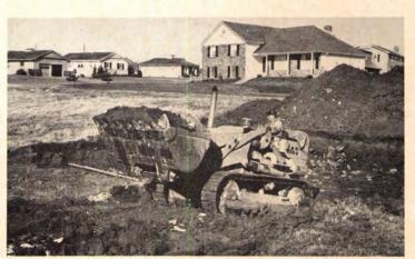
**Track-type loader** has pedal steering for increased operator efficiency, says the maker. Model 955 also includes planetary power shift transmission and automatic bucket controls. Nine bucket sizes with capacities to 23/8 cu. yds. are available. Caterpillar, Peoria, Ill.
