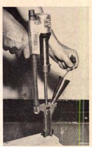
Nailer handles any bulk nail from 6d to 16d and drives as many as 50 nails per minute, according to the manufacturer. The unit weighs 7 lbs. Nails are dropped into the funnel and the trigger is pulled to operate. United Shoe Machinery, Boston. Circle 232 on Reader Service card
