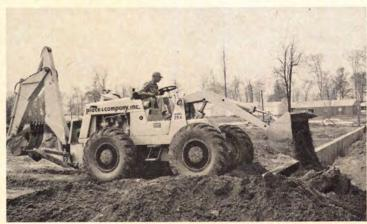
**Tractor shovel,** with four-wheel drive, has a 67 h.p. engine. The machine has a 1-cu.-yd. bucket and a 5-cu.-yd. backhoe. Also included are power steering, lights and parking brake. Clark Equipment, Benton Harbor, Mich. Circle 236 on Reader Service card.
