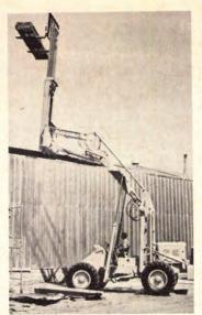
Forklift has a hydraulic forward reach to extend loads 12'7" forward without moving truck. The unit can lift 3,500 lbs. to a height of 36'. Four-wheel drive and four-wheel power steering are included. Pettibone Mulliken, Chicago.
