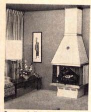
Compact fireplace has lightweight parts that slide together without special tools for quicker installation, says its maker. For safety, the hood has three layers of aluminized steel. The unit comes in three colors. Stratton & Terstegge, New Albany, Ind. Circle 149 on Reader Service card
