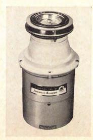
Jam-proof disposer has hammermill cutting action. Unit also has a two-lipped seal to prevent water entering the bearings. A long aluminum tailpiece simplifies installation, according to the manufacturer. American-Standard, New York City.
