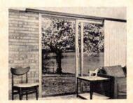
Wood patio door has double weather stripping at head and sill, and checkrail weather stripped interlock. Vertical wood sections are steel reinforced. Ball bearing wheels are said to be adjustable. R.O.W. Window Sales, Ferndale, Mich.
