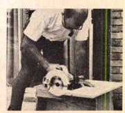
**Circular saw** is double-insulated to guard against electrical shock. Tool has a combination blade, a wrap-around handle and sawdust ejector. Model 75 has a 10 amp, 4,500 rpm motor and self-lubricating bearings. Rockwell, Pittsburgh.
