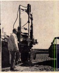
compaction, the soil engineer, Dames & Moore, drills up to 30 test cores a day to sample density of fill and to help expose hidden slurry pockets.
