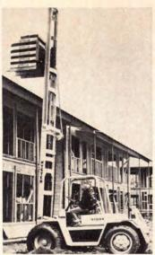
Lift truck, with a three-stage upright, can lift up to 3,100 lbs. 30' into the air. The truck has wide profile, rough terrain drive tires and a built-in towbar for highway-speed towing from job site to job site. Hyster Co., Portland, Ore.
