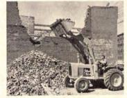
Wheel loader has power shift transmission — eight forward speeds and four backward ones. Model JD500 comes with either 1/8 cu. yd. or 11/4 cu. yd. materials bucket. Machine also has a single-lever loader control. John Deere, Moline, Ill.
