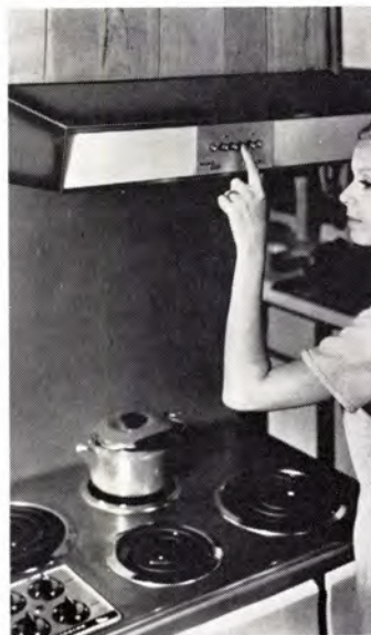
Range hood has 10" mixed-flow impellers and is arranged for vertical or horizontal discharge. The 4100 Series includes 240-sq.-in. mesh filters. Control panel has push-buttons for three speeds and switch for lights. Miami-Carey, Cincinnati.
