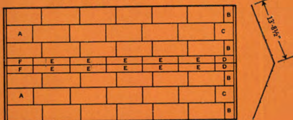
EXAMPLE OF PLYWOOD SHEATHING LAYOUT (Pitched Roof, 50' x 27'-5"; trusses 2' o.c.)
