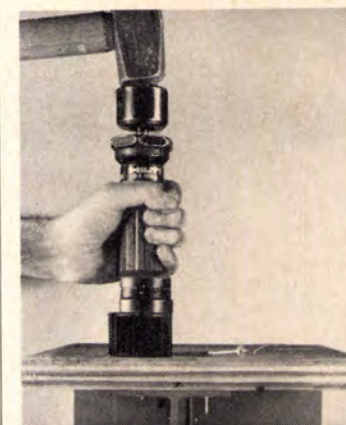
WOOD-TO-STEEL fastening ties 1\frac{1}{8} " plywood subfloor to joists.
