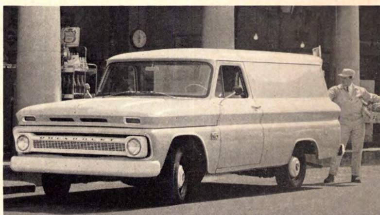
Conventional panels are available with 7½- or 10½-ft. bodies and GVW ratings to 7,800 pounds. Four-wheel-drive model with 7½-ft. body is also offered.
