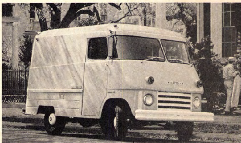
Forward-control Step-Vans offer walk-in convenience and spacious bodies up to 12½ feet long. GVW ratings go up to 10,000 lbs. on models with dual rear wheels.
