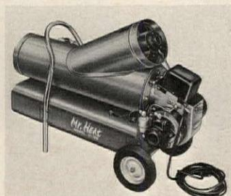
**Portable space heater** has blower intake on top of housing to provide a booster air supply. Two new models—with 100,000 or 170,000 Btu/h ratings—burn kerosene or #1 fuel oil and operate on standard 120V AC current. Mr. Heat, St. Louis. *Circle 268 on Reader Service card*
