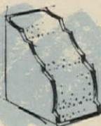
Solid, silent insulated sandwich walls have FORMICA® brand laminate interior bonded to 5/8" water impervious foam core and 1/16" melamine back-up sheet.
