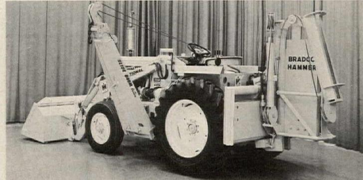
**Pipe-setter tractor** combines four tools to do the entire job: It breaks concrete (or other surface), digs a trench, lays pipe, backfills, and tamps. Hydraulic slide boom handles up to 4,500 lbs. International Harvester, Chicago. *Circle 267 on Reader Service card*
