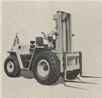
**Towable fork-lift truck**, with lifting heights to 16', incorporates a 109 h.p. engine, 13" clutch, and heavy-duty drive axles. The 14:00x20 drive tires provide broad surface contact for rough terrain. Capacity: 6,000 lbs. Champ, El Monte, Calif. *Circle 282 on Reader Service card*
