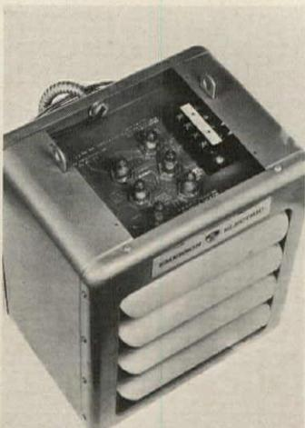
**Suspended unit heater**—with wall or ceiling brackets—comes with manual or automatic controls. Its motor is enclosed and permanently lubricated. Line includes compact 1½ to 36 kw models. Emerson Electric, St. Louis.
