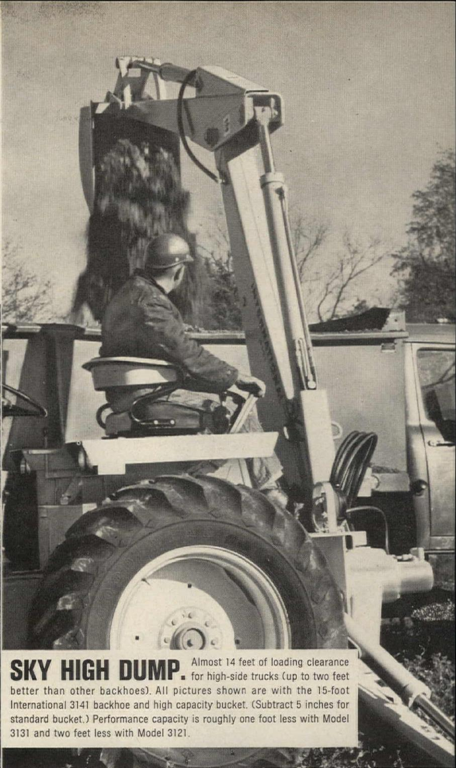
**SKY HIGH DUMP.** Almost 14 feet of loading clearance for high-side trucks (up to two feet better than other backhoes). All pictures shown are with the 15-foot International 3141 backhoe and high capacity bucket. (Subtract 5 inches for standard bucket.) Performance capacity is roughly one foot less with Model 3131 and two feet less with Model 3121.
