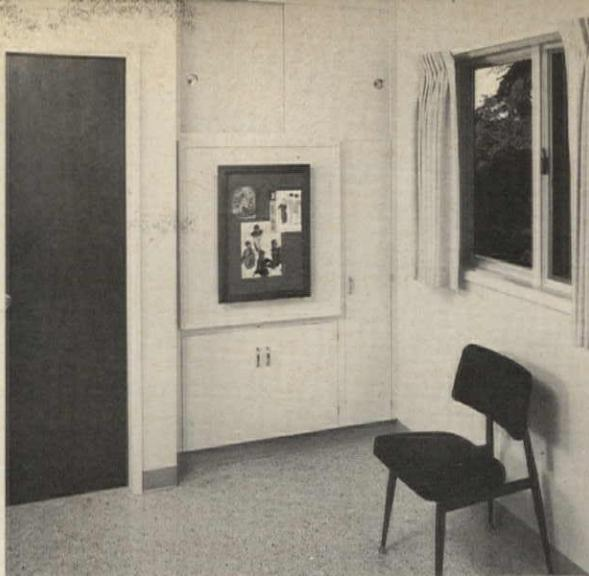
**CLOSET SEWING UNIT** fits into recess beside small bath. It includes a wall-hinged table, narrow closet for ironing board, variety of shelves and drawers, and overhead bulk storage. Builder: Jeff Ehlen, Lake Oswego, Ore.
