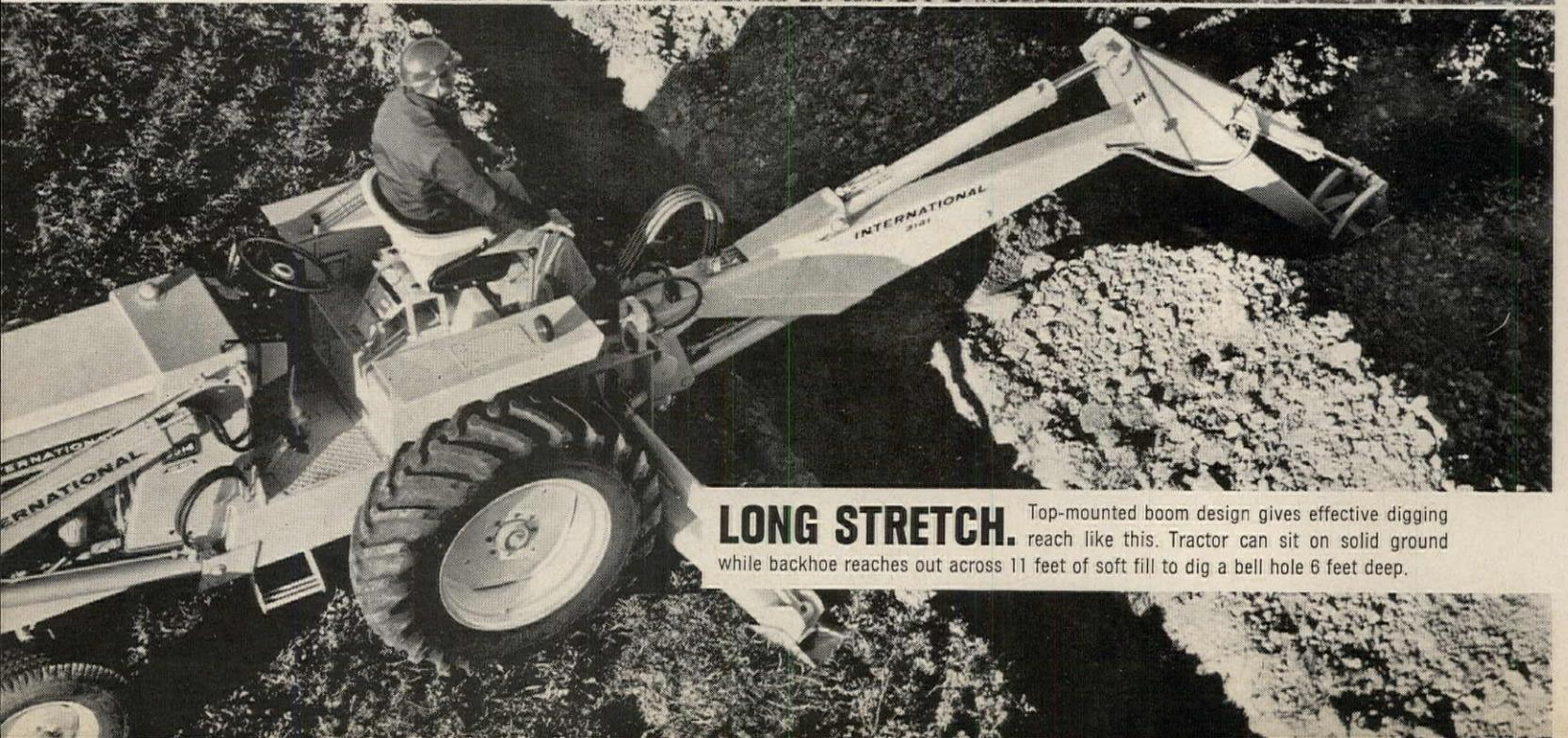
**LONG STRETCH.** Top-mounted boom design gives effective digging reach like this. Tractor can sit on solid ground while backhoe reaches out across 11 feet of soft fill to dig a bell hole 6 feet deep.
