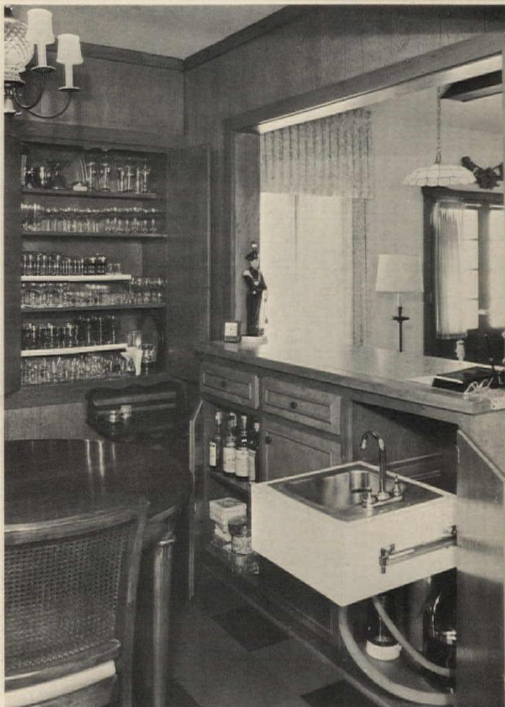
**ROLL-OUT BAR SINK**—mounted on drawer slides and plumbed with hoses—is concealed inside doors when area behind bar is used for dining. Builder is Morris Franklin.
