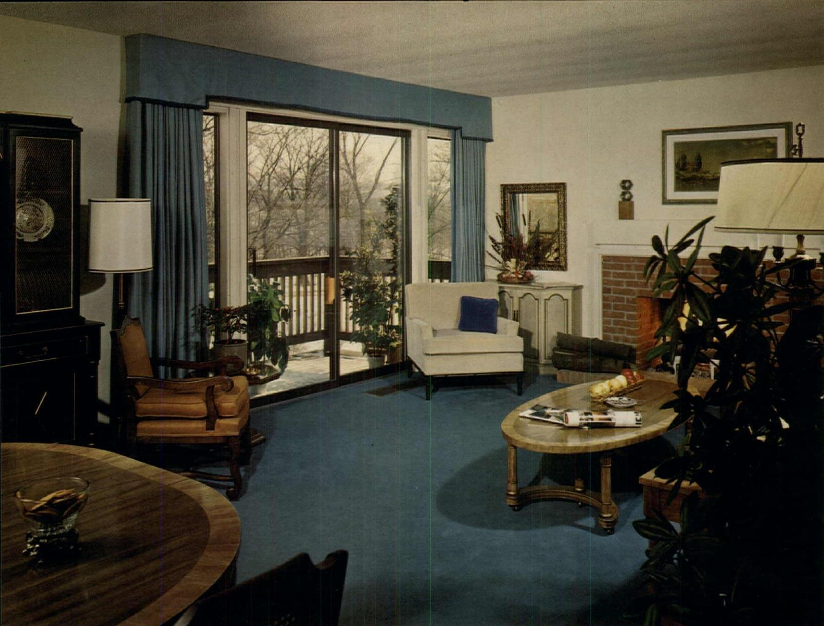
**SLIDING GLASS DOORS** open from living room to balcony of Ethan Allen model. Double-glazing and extra register in front of door minimize cold drafts.
