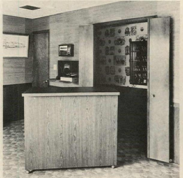
**ROLL-OUT COUNTER.** with shelves on one side, doubles as bar and portable buffet. Stephens builds his bar alcove into family-room wall and closes it in with flush bifolds.
