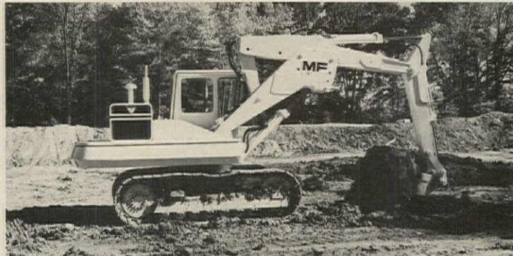
**Hydraulic excavator** with bucket capacity of 3/8 to 1/2 cu. yds. digs up to 16' deep (larger model digs to 19 1/2'). Wide range of optional equipment includes reversible buckets, clamshells and crane jibs. Massey-Ferguson, Akron, Ohio. Circle 215 on Reader Service card
