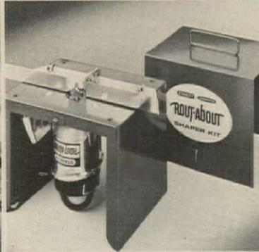
**Compact shaper kit**—with straight and circular guide, adjustable fence and straight bit—turns portable router into an inexpensive shaper. Router locks into base of carrying case (left), which becomes a 6"x8" table. Stanley, New Britain, Conn. Circle 213 on Reader Service card
