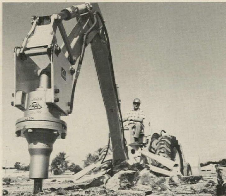
**Hydraulic impactor**—shown teamed with a tractor-backhoe-loader—breaks pavement (above), tamps backfill, and drives posts or pilings. It can be installed quickly in place of the backhoe bucket. Ford Motor Co., Birmingham, Mich. Circle 217 on Reader Service card
