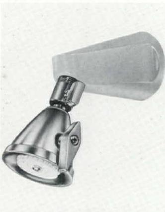
**Non-scald showerhead** is made of triple chrome-plated brass with interior components of thermoplastic NORYL. Available with fixed or adjustable spray patterns, volume control, fixed-quantity flow restrictor. Symmons Engineering, Boston. Circle 251 on Reader Service card
