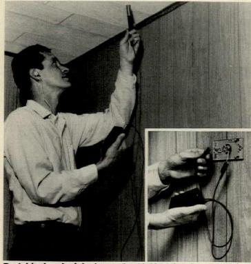
**Portable break detector**—a hand-held probe plus transmitting/ receiving unit—pinpoints breaks in hidden or inaccessible wiring to within 1" and through material as thick as 6". Unit operates on 9-volt battery. Systems Research, Portland. Circle 210 on Reader Service card
