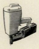
Drives 16d nails with one blow. Powerful, fast nailing of box, sinker, common and screw-type nails— 4,000-5,000 an hour, including reloading time. Cartridge loading. Tool weighs only 11 pounds. Nails conform to Federal Specification FF-N-105a, Interim Amendment-2, April 7, 1964.
