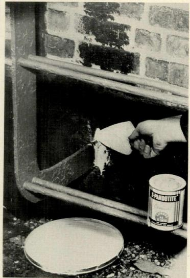
**Expansive cement**—expansion is from .002" to .004" per cu. in. can be used both to repair cracks and to anchor materials including metal. Cement does not shrink or crack and is unaffected by water. X-Pando, Long Island City. *Circle 200 on Reader Service card*
