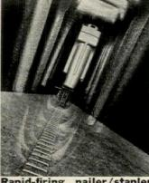
**Rapid-firing nailer/stapler** drives up to 12 fasteners per second, depending on length of fastener and type of wood. The tool can be set at a high, medium or low speed by adjusting the metering bolt in the cap. Spotnails, Rolling Meadows, Ill.
