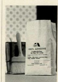
Water-mix adhesive, for vinyl and other nonporous wallcoverings, is nonstaining and permits slippage for pattern matching. Adhesive is dry-packaged in bags of 1, 2 and 5 lbs.; 1 lb makes 13 pints of paste. Evans Adhesive, Columbus, Ohio.
