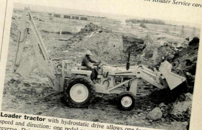
**Loader tractor** with hydrostatic drive allows one-foot control of both speed and direction: one pedal controls forward travel, a second controls reverse. Drive is optional on two loader tractors and industrial tractor. International Harvester, Chicago. Circle 221 on Reader Service card
