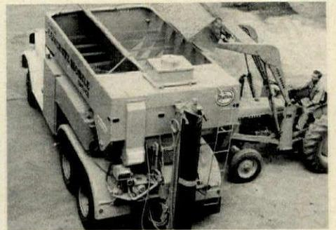
**STORAGE COMPARTMENTS** for sand and aggregates are loaded from top. Cement and water are kept in sealed tanks. Materials are proportioned, mixed and metered from central control panel (below) at rear of truck.
