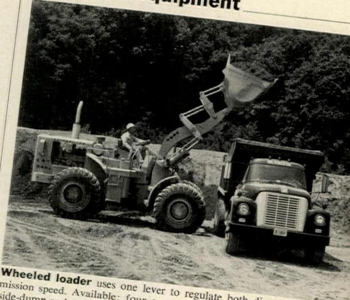
**Wheeled loader** uses one lever to regulate both direction and transmission speed. Available: four general-purpose buckets as well as rock, side-dump and multi-purpose buckets and a rear-mounted ripper-scarifier. Caterpillar, Peoria, Ill. Circle 218 on Reader Service card
