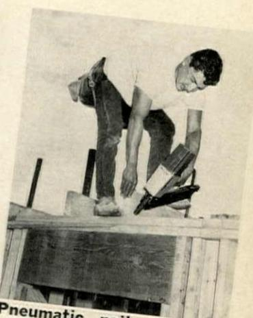
**Pneumatic nailer** drives a range of nails from 6- to 16-penny, prepackaged in clips that load easily into tool's magazine. Nailer has a lightweight aluminum body and can be used in a vertical, horizontal or overhead position. International Staple, Butler, Pa. Circle 220 on Reader Service card
