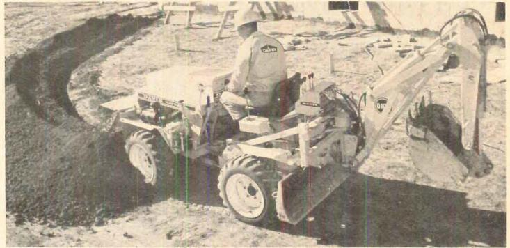
**Four-wheel-drive trencher** has single lever control, will dig from 18" wide and 24" deep to 4' wide and 60" deep at up to 1500' per hour. Also available: a backhoe that digs up to 8'4" deep with separate controls. Davis, Wichita, Kan. *Circle 217 on Reader Service card*
