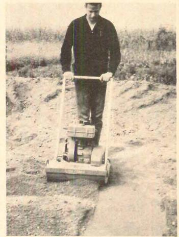
**Earth compactor** with 23" wide steel plate packs 4,200 lbs. of force at up to 4,400 vpm, operates at 370 lbs., travels at up to 90' per min. over soft or rough ground. Choice of three manufacturers' 6 hp engines. Kelly Industrial, Beresford, S. Dak. *Circle 219 on Reader Service card*
