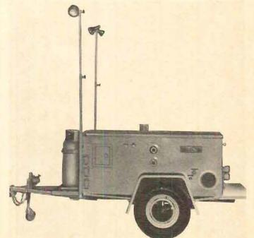
**Mobile power unit** supplies electric power for tools or floodlights and provides heat from a flameless 45,000 BTU hot water furnace. The 6500-watt generator operates on gas or propane. All steel body is 6' x 4' x 30" deep. Holtkamp, Centralia, Ill.
