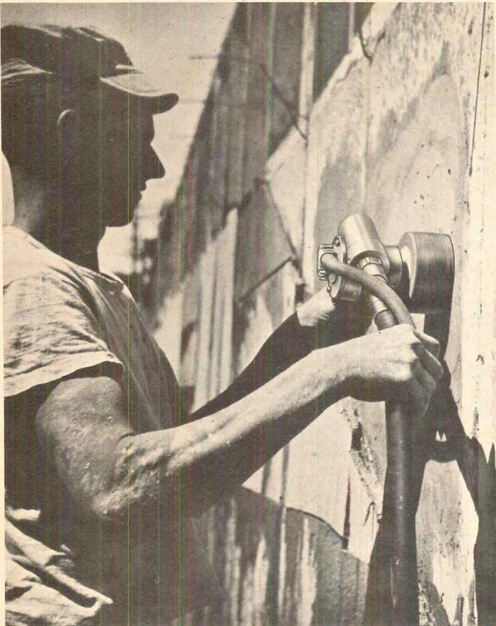
**Concrete grinder** has an 8' or 12' flexible shaft designed to reduce the weight held by the operator, is powered by a  $\frac{3}{4}$  hp electric motor or a 3 hp gas engine, can be used for dry grinding or wet rubbing. Stow, Binghamton, N.Y. *Circle 214 on Reader Service card*
