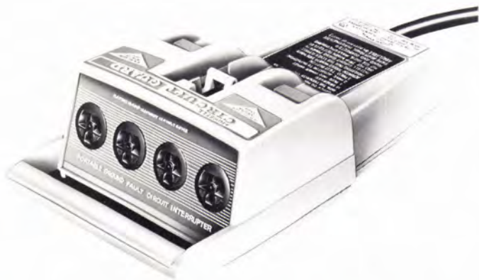
Circuit interrupter is lightweight, plugs into any outlet. Portable tools plug into the four 15- or 20-amp. outlets which interrupt deadly line-to-ground faults too minor to activate usual breakers. Harvey Hubbell, Bridgeport, Conn. Circle 214 on Reader Service card
