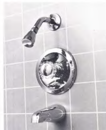
Nonscald faucet has just one moving part, balances pressure to maintain even water temperature despite drains on supply lines. Design features a single-handle control—either a dial, as shown, or a lever—in 14 styles. Delta, Taylor, Mich.
