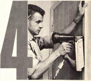
Fast, mar-free interior trim work . . . is easy with Duo-Fast Brad and Finish Nailers. Automatic countersinking eliminates nail-setting. Color brads are available to match pre-finished trims. Duo-Fast has models to cover the complete range of brads and finish nails.
