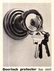
ball in the tumbler that allows one key to operate during construction. A second key allows ball to be withdrawn by a magnet, so only the third—homeowner's—key will operate lock. Weslock, Los An-
