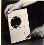
Radiant ceiling installs like any drywall panel. Insulated resistance cable is buried in 5%" gypsum board, heats to about 125° when connected to 240-volt wiring. This gives a surface temperature of 100°. National Gypsum, Buffalo, N.Y. Circle 360 on Reader Service card
