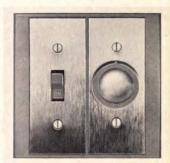
Dimming switch is the first 277-volt fluorescent dimmer that will control up to twenty 40-watt fluorescent bulbs. Needs no auxiliary ballasts or remote dimming sections. Solid state controls, for single- or three-phase systems. Lutron, Coopersburg, Pa.
