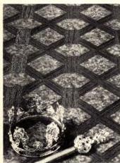
Sheet vinyl has the look of inlaid marble combined with wood to set off this 6'-wide flooring. An interlayer of vinyl foam muffles sound and increases resiliency. An asbestos backing allows installation on, above, or below grade. GAF, New York City.
