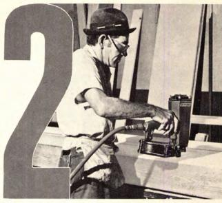
Component mass production ... needs tools like the Duo-Fast IN-123 to match the efficiency of in-plant or shed construction. Many on-site uses too. Fed from a coil of 300 nails, the IN-123 handles regular, ring and screw shanks, from  $1\frac{1}{4}$ " thru  $1\frac{7}{8}$ ". Built-in safety mechanism.
