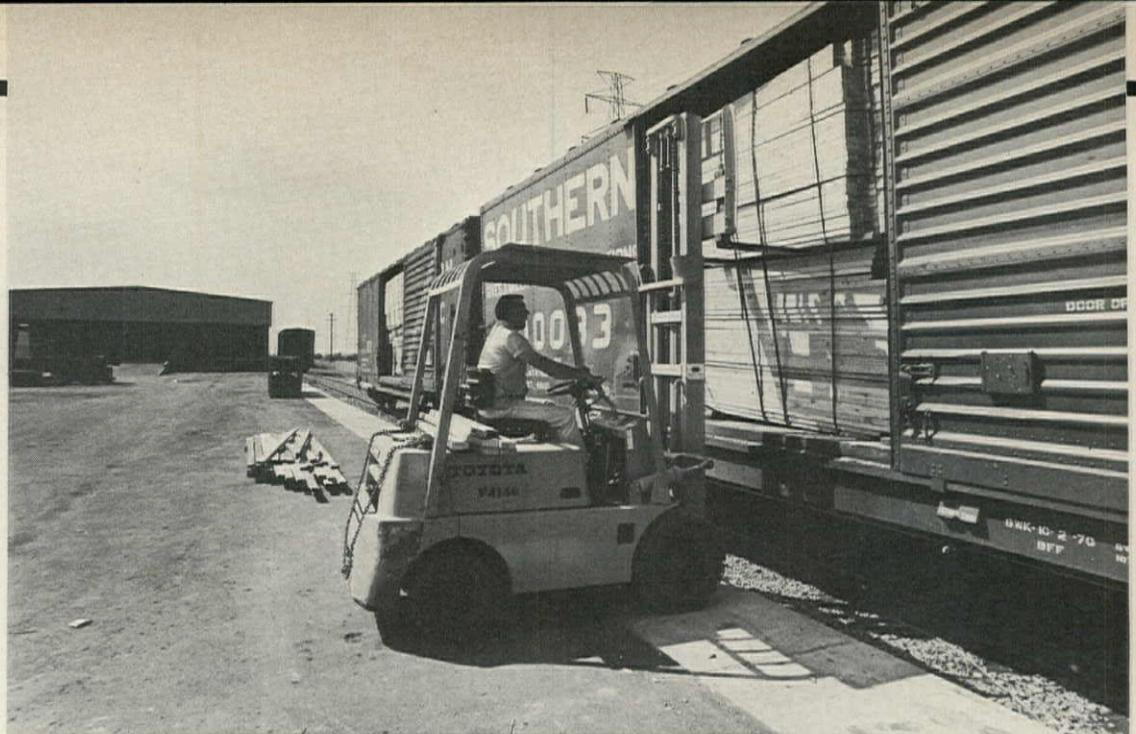
**1** Lumber is taken off boxcar with forklift. One man can unload a carload of studs in about 30 minutes; formerly, done by hand, it took four days.
