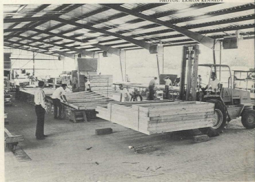
④ Interior panels are picked up for moving to staging area. The company plans to install overhead cranes at the ends of the production lines.
