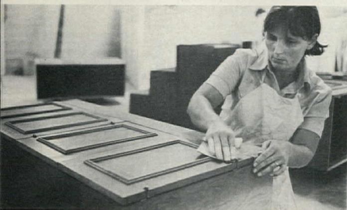
7 Cabinets are hand-sanded between sealing operation and subsequent lacquering.
