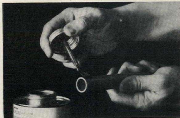
Then brush cement on the outside of the tubing. Notice how easy it is to handle. Tubing made of hi-temp Geon resists moisture, oil, corrosion, acids, alkalis and other chemicals.
