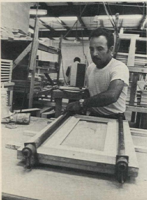
3 Arch material, cut in previous operation, is assembled with power stapler and glue.
