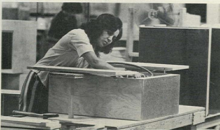
5 Doors are installed on overhead kitchen cabinet with air-powered screwdriver.
