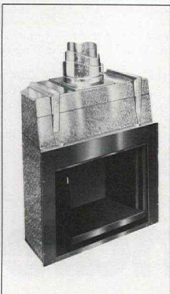
Pre-fab wood-burning fireplace system with zero clearance to combustibles has a companion masonry face and hearth set. Fireboxes have one-piece steel-reinforced cast refractories that will not break. Ashes and sparks are contained within the firebox by a special lip and an overlapping screen. Superior Fireplace, Fullerton, Calif.
