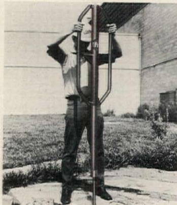
Breaking tool delivering 80 ft./lbs. of energy at impact point, easily demolishes concrete, asphalt and rock. The lightweight portable tool can be used anywhere a sledge is called for or to drive posts, tube anchors, pipes and stakes. Designed for safety and speed, impact end of the breaker never loses contact with the object being demolished or driven. A push on the handles starts the pounding action, then a spring loaded mechanism lifts the driving unit. Kelley, Buffalo, N.Y.
