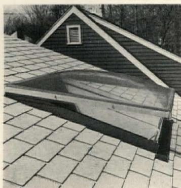
**A weatherproof Plexiglas skylight** helps solve ventilating as well as lighting problems. Offered in 6 sizes up to 4' square, units come complete with curbing, screen and copper flashing suitable for use with shingle or flat roofing. Available with manual control pole or motorized electrical operation, units are leakproof, dustproof, draftproof, self cleaning and free from condensation. Ventarama Skylight, Port Washington, N.Y. CIRCLE 211 ON READER SERVICE CARD
