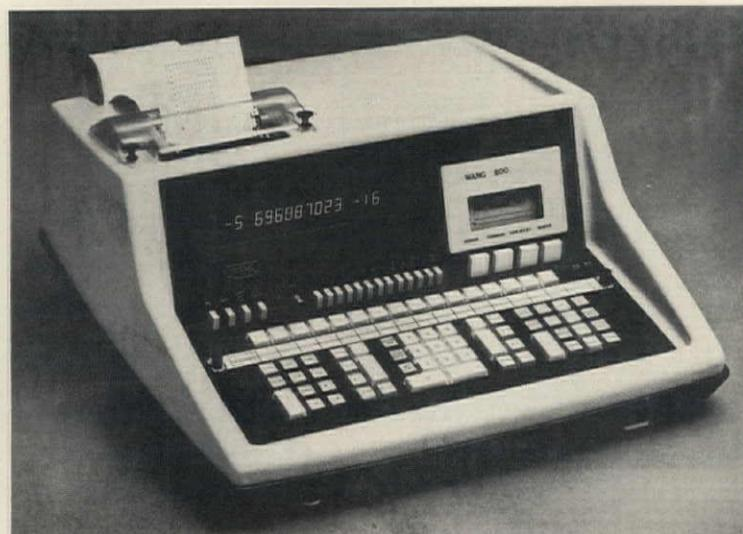
**Electronic calculator** features algebraic programming, making it possible to enter formulas as they are written. Instead of using standard machine language, the unit solves
