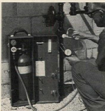
**Leak detecting kit** for piping eliminates the necessity of on-site air compressors which provide the necessary pressure source. After both ends of the pipe are shut, a pressure test line is inserted into the inspection connection of the gas line shut-off valve. The pressure gauge in the kit indicates the level of charge and holds at the highest reading indication. If a leak is present, a second pointer moves lower. Cyclonics, Medina, Ohio. CIRCLE 233 ON READER SERVICE CARD
