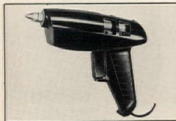
**Electric glue gun** has trigger mechanism that feeds solid hot-melt glue stick into unit and controls the flow of liquid glue applied to a surface. A factory set thermostat assures consistent glue melting and eliminates manual control of temperature. USM Corp., Reading, Pa.
