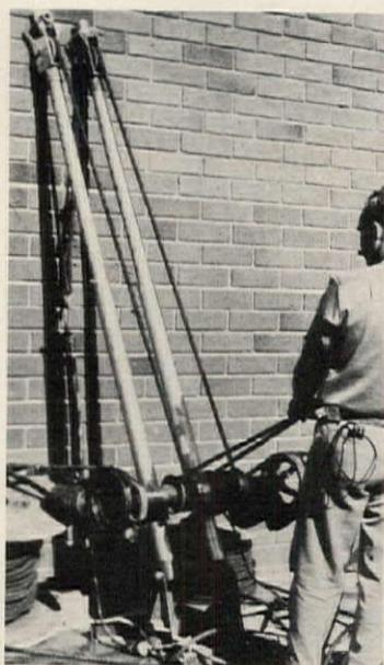
Cable puller can be adapted to use two lines for double pulling power. Tool, which can be operated by one man, pulls up, down and horizontally while standing on the floor. Weighing only 53 lbs., the puller features a telescoping shaft with 3" adjustments up to 9'. Gebo Tool & Equipment, Van Nuys, Calif.
