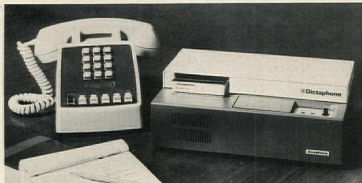
**Automatic answering system** answers the telephone and gives the caller a prerecorded message which can run from 20 sec. to 3 min. The compact unit can be connected to
