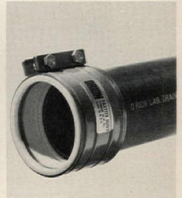
**Joint fittings** for use with waste piping systems eliminates the heat fusion process for connecting the piping. The only tools needed to assemble the fittings are a tape measure, a tube cutter and a torque wrench, reducing installation time. Orion Fittings, Kansas City, Mo. CIRCLE 231 ON READER SERVICE CARD
