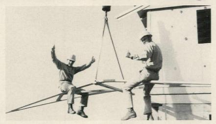
Even with the racking weight of a full-grown man on each side, this Fink truss joint won't give. It's fastened with Bostitch Clinch Nails – the heart of a unique truss system that combines the proven strength and durability of nail-on truss plates with the speed and low cost of simple, compact air guns.
