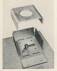
Post base clip aids in beam erection, making post positioning easy even when bolts are out of line. The adjustable two-piece clip consists of a base cover of 16-gauge zincplated steel and a support plate of 11gauge galvanized steel. The cover, equipped with weep holes to prevent moisture build-up, has a special finish that resists weathering and holds paint. Engineered for use with 4"x4" posts, the clips are termite resistant and rotproof. Panel Clip, Farmington, Mich.
