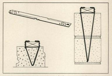
Framing device, which anchors wood sills to either concrete or masonry-unit foundations, replaces the conventional bolt anchor in most installations. The 18% "-long, 1"-wide zinc-coated steel unit can
