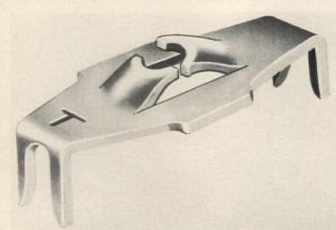
Self-locking Tinnerman wood anchors speed fastening of plywood panels by eliminating spanners and lock washers. The anchor is placed over a drilled hole and tapped into the wood. A screw is then inserted into the hole and turned until tight. Clips grab the screw and hold it securely. Anchor can be use with .028" to .031" plywood. Engineered Fasteners, Cleveland, Ohio CIRCLE 225 ON READER SERVICE CARD
