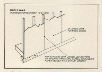
APA Single Wall as combination siding-sheathing completely eliminates one application step.
