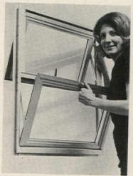
Aluminum vent windows can be opened to any position and held by an adjustable friction stay arm. The 15/8"-deep units accept glass from 1/8" to 1/2". White bronze handles lock the vents into closed positions. Amarlite/Anacondia, Atlanta, Ga. CIRCLE 231 ON READER SERVICE CARD
