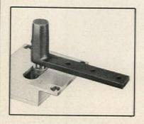
Heavy-duty rack and pivot hinge is structured to support doors up to 150 lbs. The hinge, which is designed to eliminate the need for rounded door edges, permits installation with close tolerance fit and concealed hardware. Heavygauge metal and bottom pivot support provide extra floor anchorage. Gear housing can be cement-set. Hager Hinge, St. Louis, Mo. CIRCLE 233 ON READER SERVICE CARD
