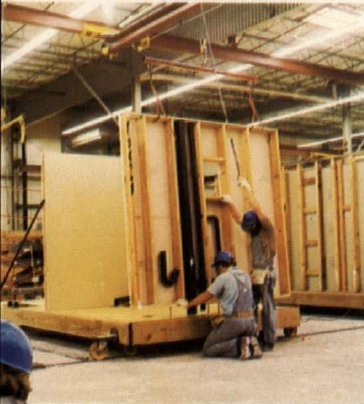
Final stages of production add cabinets, appliances, mechanical hook-up and testing, interior wall finishing and wrapping for shipment via truck and rail as far as 1,200 miles.
