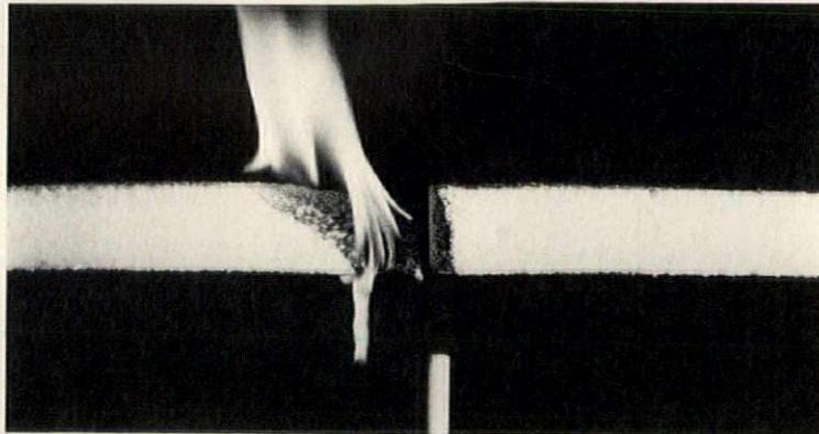
Polyurethane foam flames up, left, when lit by gas torch in test by GAF Corp., New York City. But GAF claims that if its fire-retardant monomer, dibromobutenediol, is injected into the same foam, the foam will then extinguish itself, as shown at right.
