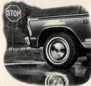
**10** Front disc brakes are standard on all '74 Ford pickups with 2-wheel drive.
