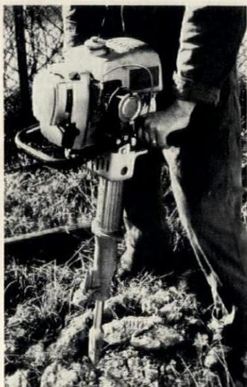
Self-contained utility breaker meets the demands of extended use under punishing operating conditions. The gasoline-driven tool is equipped with a 5 cu. inch, 2.6 hp two-cycle, air-cooled engine. Breaker meets OSHA requirements and features a sound muffler to hold down noise level. Wacker, Milwaukee, Wis.
