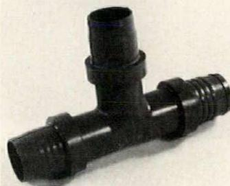
**Water line fittings**, designed specifically for use with polybutylene flexible tubing, make installation and service of mobile home potable-water lines simple. Solvents, cements and joint-cleaning are unnecessary. Fittings, in coupling or tee configurations, engineered for on-site or factory assembly, use a single-crimp repetitive connection technique. Amp, Valley Forge, Pa.
