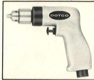
**Pneumatic drill**, with a pistol handle grip and compact 3 hp rotary vane motor, is designed for minimum operator fatigue. Lightweight, heavy-duty tool has an optional overhead hose that holds sound level at 75 decibels. Drill features a rear-exhaust and an adjustable speed regulator. Dotco, Hicksville, Ohio.
