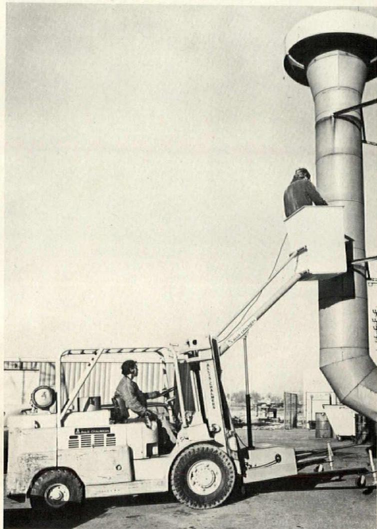
**Molded plastic cab** is offered as standard for the 500 lb. capacity maintenance-man attachment for lift trucks. The three layer laminated unit, measuring 25"x32"x42", has an open front for access to work. The fire-resistant cab is fastened to the boom and can be easily and quickly removed. Allis-Chalmers, Milwaukee, Wis. CIRCLE 257 ON READER SERVICE CARD
