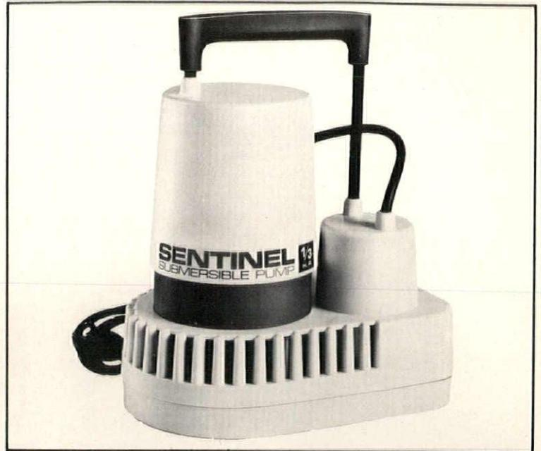
Low-cost, submersible sump pump operates on the vortex principle—a polypropylene impeller spins at 3,100 rpm creating a whirlpool that passes lint and solids without clogging the mechanism. Top-suction pump is actuated by a rising water level. The lightweight unit has a housing of polycarbonate instead of metal. Penberthy, Prophetstown, Ill. CIRCLE 241 ON READER SERVICE CARD
