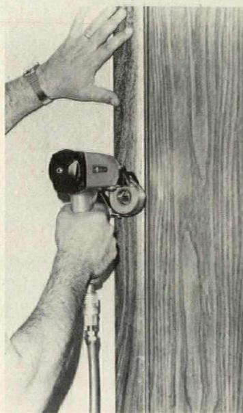
**Automatic fastener, Spotbradder™**, helps reduce downtime and speeds up production. The lightweight 3 lb. unit carries a 925-load coil cartridge of Spotbrads™. Cartridge snaps on instantly permitting almost continuous operation of the tool. Spotbradder™ drives 18-gauge brads from 3/4" to 1" in length and 18-gauge pins from 3/4" to 1 1/2" long. Spotnails, Rolling Meadows, Ill.
