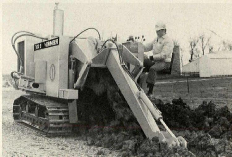
**Heavy-duty, track-mounted trencher** digs 6' deep and up to 24" wide with a 150,000 lb. test, multi-speed digger chain. Low-maintenance gasoline-powered unit features formed plate heavy construction and balanced design. It travels on wide, high-flotation, springloaded tracks mounted on seven-track rollers. Vermeer, Pella, Iowa. CIRCLE 248 ON READER SERVICE CARD
