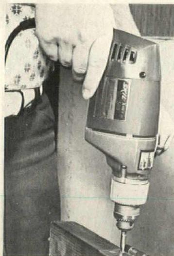
Electric hand tool combines the functions of the drill and the hammer drill. The "599 Xtra-tool" serves as a basic 3/8" drill powered by a 1/3 hp motor, a high frequency impact tool for chiseling, scraping and gouging and as a hammer-drill, particularly efficient in drilling concrete, brick and masonry. Skil, Chicago.
