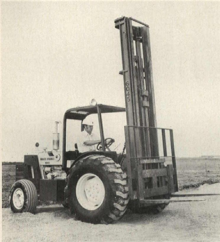
**Rough terrain forklift**, with a 6,000 lb. lift capacity, is powered by a 63.7 hp Ford industrial tractor. Optional masts, providing lifting heights to 30'6", are available. Heavy-duty unit features a quick drive train disconnect that allows the forklift to be towed at road speeds with the drive train disengaged. BadgerDynamics, Port Washington, Wis. CIRCLE 254 ON READER SERVICE CARD
