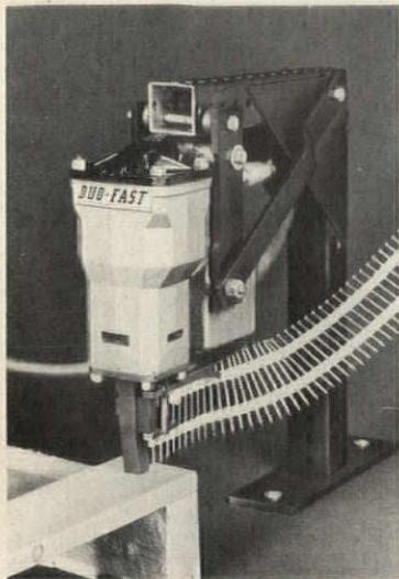
**Rapid-firing pneumatic nailing head** is available for custom mounting in equipment designed for automated woodworking assembly application. The unit drives 4" and 3 1/4" coated nails with either smooth or screw shanks. Tool is adaptable to remote firing by hand or foot switch. Duo-Fast, Franklin Park, Ill.
