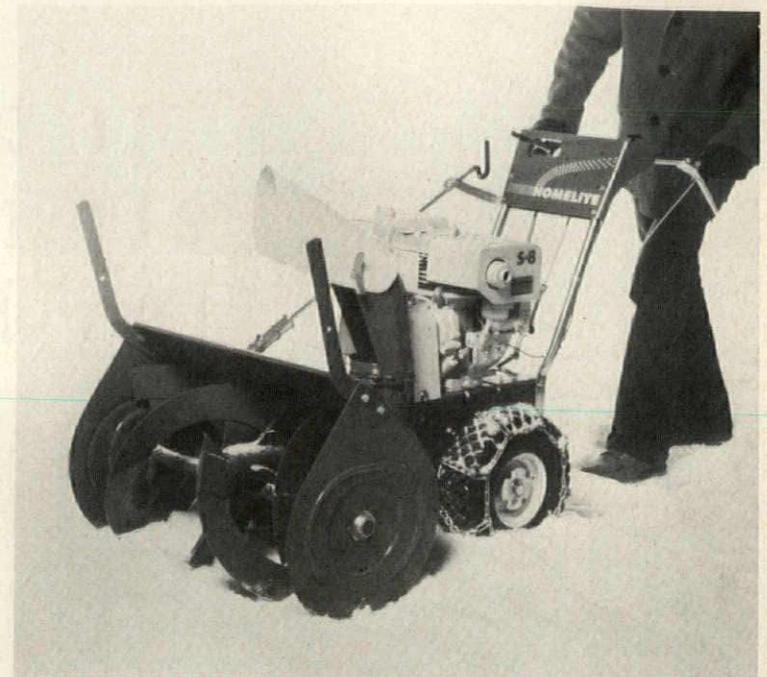
**Two-stage 8 hp snowblower** is equipped with a single cylinder, air-cooled, four-cycle Briggs & Stratton gasoline engine. Unit, with three forward gears and one reverse, features a built-in differential for maneuverability and can be locked for positive two-wheel traction. Blower has a discharge radius of 270°. Homelite, Portchester, N.Y. CIRCLE 249 ON READER SERVICE CARD
