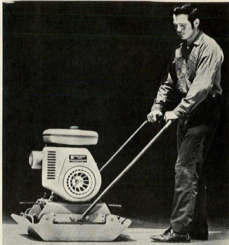
**High-speed reversible plate compactor** compacts granular and cohesive soils to a depth of 30". A 10.5 hp Wisconsin-Robbin gas engine delivers 4,000 blows per minute with a 6,000 lb. force per blow. Unit, with an 18" sq. plate, features a "Touch-toe" control and swing-over handle. J.I. Case, Racine, Wis.
