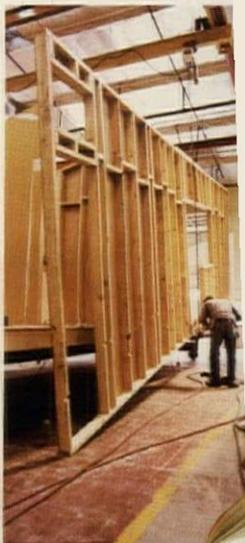
So it was a simple and logical step for Levitt to expand its California mobile home business into the sectionalized housing market. The same production line produces a mix of mobile and sectionalized homes at the rate of five “floors” per day.
