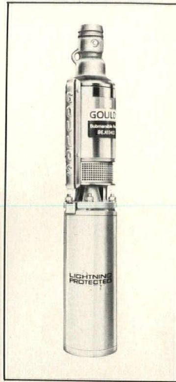
Line of two-wire submersible pumps consists of 31 models suitable for 4" and larger wells. All are powered by Franklin Electric's "Super Stainless" motors with built-in lightning arrestors. Units feature bronze and stainless steel construction, water lubricated bearings and flat bowl design. Goulds, Seneca Falls, N. Y.
