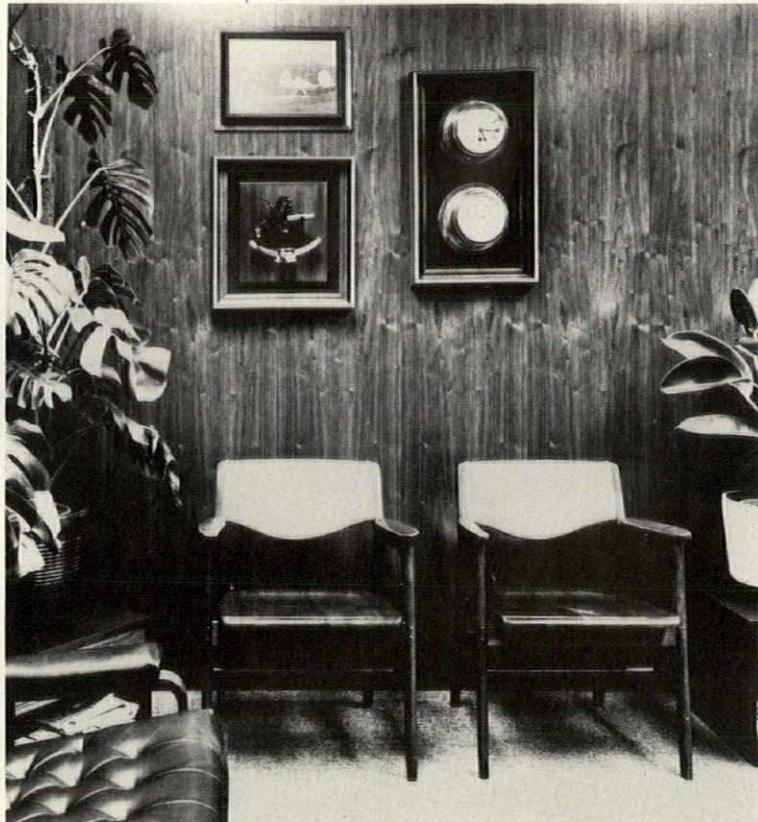
Architectural wood veneer panels, "Tech-guard," can be easily converted from Class III to Class II flamespread ratings. Unfinished panels are installed, treated with clear "Flamort WC" fire retardant and finished in the appropriate woodtone. Tech-Sales, Portland, Ore. CIRCLE 218 ON READER SERVICE CARD
