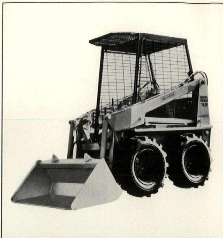
Compact Uni-Loader "Model 1830" features hydrostatic four-wheel drive and a water-cooled, four-cylinder gasoline engine. The width is only 54" and height to the top of the ROPS canopy is under 7'. A choice of buckets is offered. J.I. Case, Racine, Wis. CIRCLE 263 ON READER SERVICE CARD
