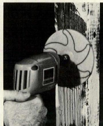
Paint removing disc, "Paint-Z-Off", is designed with tiny saw teeth that rub down to original wood in seconds. Unit, which fits standard drills, leaves a lightly textured surface ready for sanding, painting or staining as desired. Samuel Cabot, Boston.
