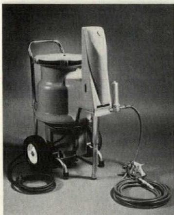
Portable airless sprayer can support one gun with a .031" orifice or two guns with .021" orifices. The heavy duty rolling unit delivers a continuous output of 1.0 gpm at a maximum working pressure of 2700 psi. Graco, PDC Div., Minneapolis, Minn.
