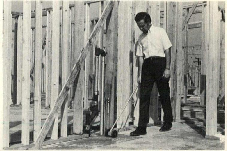
**Measuring wheel** contains a precision counter that automatically records distances in inches and feet up to 1,000 feet as the operator walks along. Unit can subtract as well as add and features a pushbutton return. Rolatape, Santa Monica, Calif.
