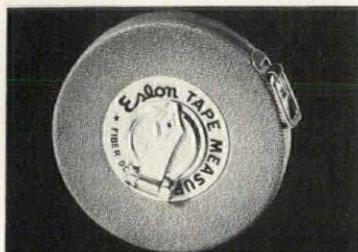
Rustproof fiber glass tape measure is calibrated in inches on one side and meters on the other. The 50'-long, 5/8"-wide tape, will not shrink or distort and is fully retractable. Unit, housed in a burnt-umber, grained steel case, features a belt loop for easy carrying and ready access. Sekisui Products, Linden, N.J.
