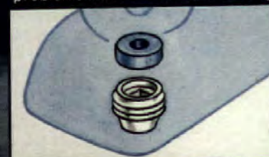
Chloroprene polymer bib washer and nickel plated replaceable seat assures long life
