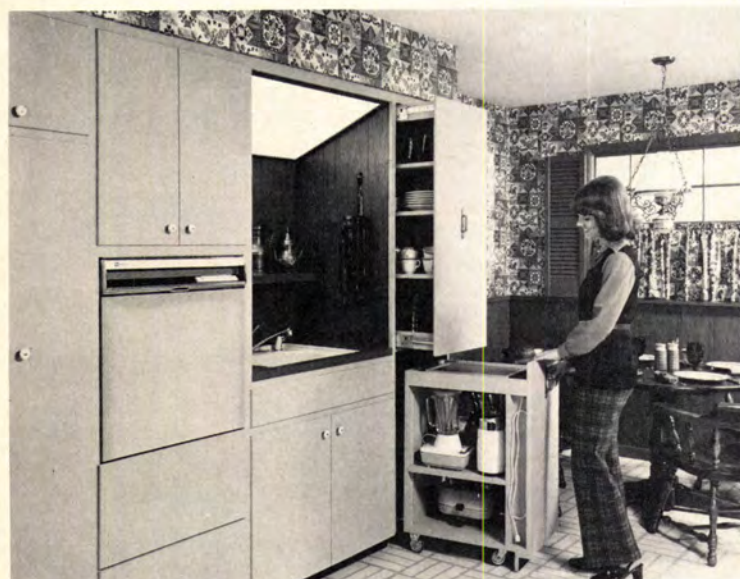
Dishwasher (above) can be built in 18 inches from the floor to simplify loading and unloading. A cabinet panel directly below the appliance comes off for easy servicing. The kitchen shown also includes a roll-around appliance cart equipped with a warming tray on the top surface. Maytag, Newton, Iowa.
