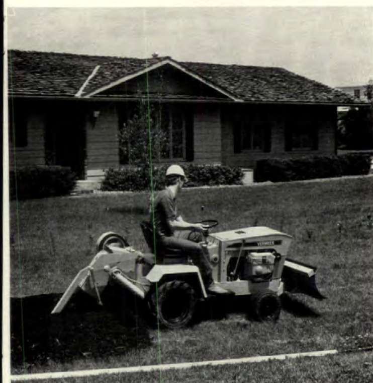
Compact trencher, "M-220," is powered by an Onan air-cooled, 19 1/2 hp engine. The easy-to-handle unit has a maximum digging depth of 36" at 4"-6" widths. A vibratory plow can be mounted in place of the trencher to install service lines. Vermeer, Pella, Iowa, CIRCLE 258 ON READER SERVICE CARD
