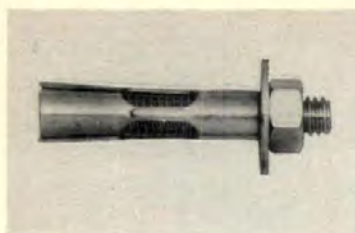
Medium-duty anchoring device, "Parasleeve" (left), is for fastening in masonry material. Preassembled unit has a zinc-plated steel sleeve over a hardened, threaded and tapered steel bung. Easy-to-install anchor requires no special tools. USM, Shelton, Conn. CIRCLE 250 ON READER SERVICE CARD
