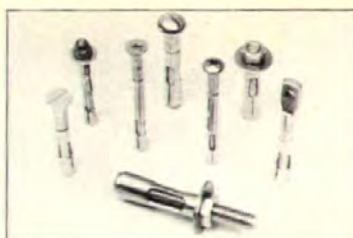
Medium-duty anchoring device, "Parasleeve" (left), is for fastening in masonry material. Preassembled unit has a zinc-plated steel sleeve over a hardened, threaded and tapered steel bung. Easy-to-install anchor requires no special tools. USM, Shelton, Conn. CIRCLE 250 ON READER SERVICE CARD
