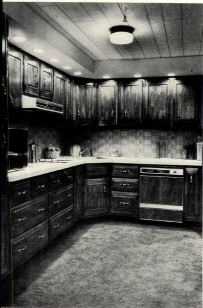
Traditionally styled cabinets (above), part of the "Rondelle" line, have rigid, mortised and tenoned construction. Units, available in a range of sizes, have metal-lined bread drawers and behind-the-door roller-mounted storage bins. Brammer, Davenport, Iowa. CIRCLE 210 ON READER SERVICE CARD
