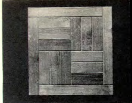
Architectural hardwood flooring, "Lincoln" (above), features slatted center and log-cabin corners. Individual 3/4" T&G solid pieces preassembled to form easy-to-install 24"-square sections. Flooring is available in a wide range of woods. Wood Mosaic, Louisville, Ky. CIRCLE 236 ON READER SERVICE CARD
