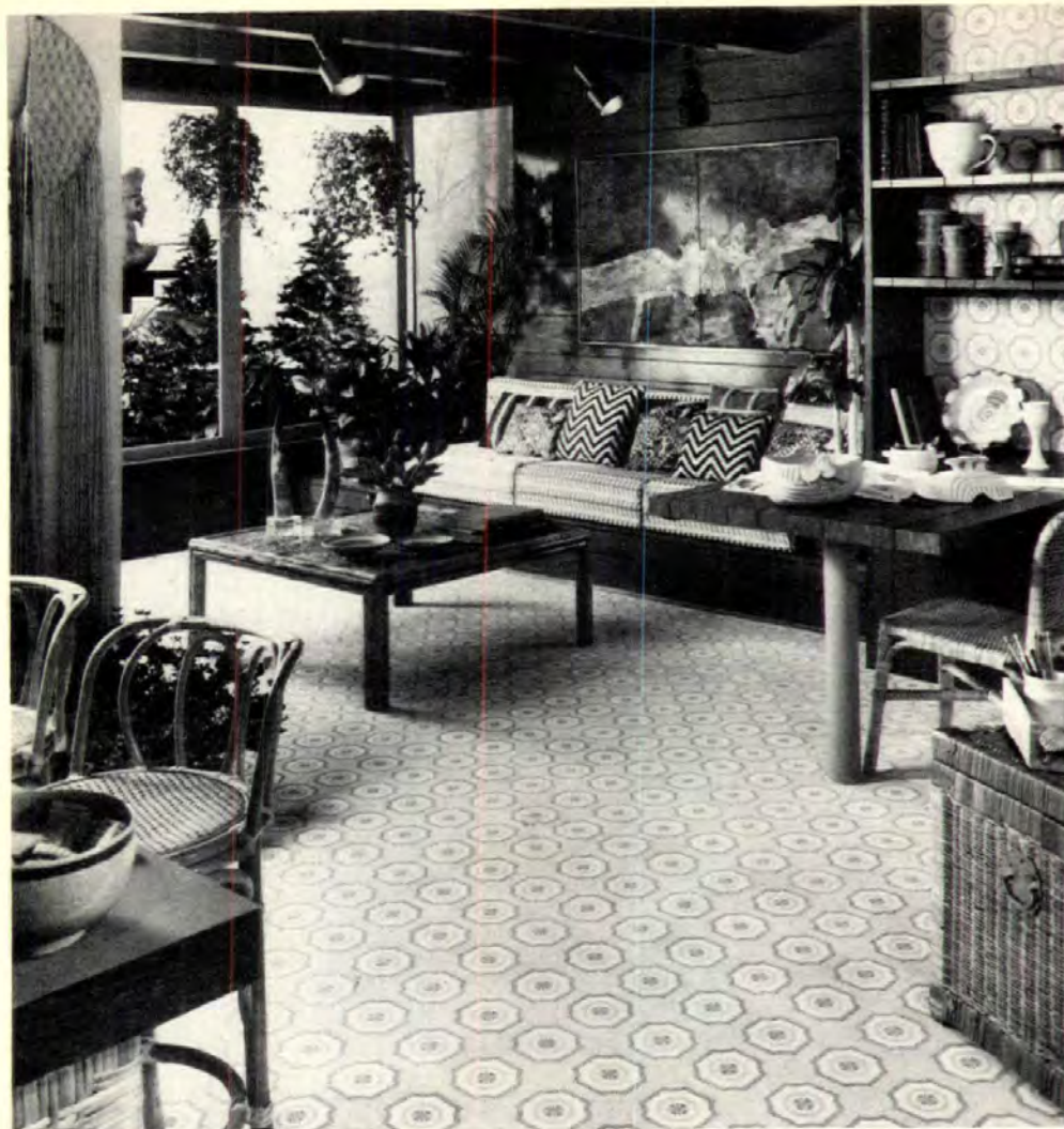
Vinyl asbestos tile, "Arlington" (above), has an embossed surface that helps hide scuffs, heel marks and subfloor irregularities. Prewaxed tile in geometric pattern can be installed directly on concrete slab or over wood subfloors. A choice of four colors is offered. Azrock, San Antonio, Tex. CIRCLE 232 ON READER SERVICE CARD
