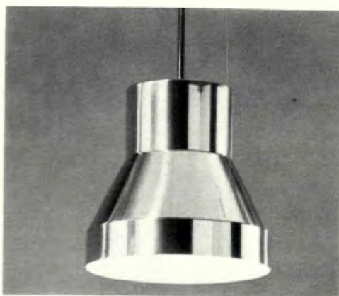
Outdoor luminaire (above) features a diffuser in a champagne glass shape. Offered in clear, translucent, bronze or smoked glass, unit can be mounted directly to a 1½" diameter tenon or with a cast-aluminum slipfitter, set onto poles of larger diameter. ITT Landmark, Southaven, Miss. CIRCLE 226 ON READER SERVICE CARD
