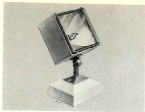
Outdoor lighting fixture, "Light Block" (above), features a precast concrete pad with an integral cast-aluminum splice box. Easy-to-install block is equipped with two bend-out wire loops which can be spiked into loose soil or anchored to a wire form. Keene Lighting, Union, N.J. CIRCLE 223 ON READER SERVICE CARD
