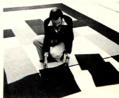
"Tretford Carpet" tiles (below) permit design versatility. The fusion-bonded, PVC-backed dimensionally stable tiles will not ravel at the edges and are suitable for loose-laid and glued-down installations. Eurotex, Philadelphia, Pa. CIRCLE 234 ON READER SERVICE CARD
