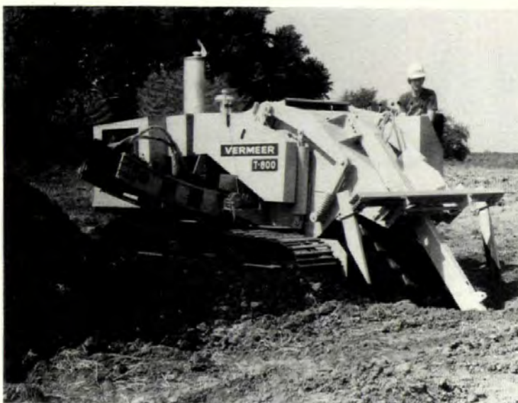
Heavy-duty trencher, "T-800" (above), digs down to 8' with trenching widths up to 36". Low-silhouette, crawler-type unit features double-digging chain system, each chain having 150,000 lbs of tensile strength. Vermeer, Pella, Iowa. CIRCLE 245 ON READER SERVICE CARD
