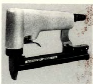
Pneumatic tacker, "Model T26-20" (above), is suitable for fastening insulation. The staple legs are automatically turned outward to clinch under or inside the work. Unit features simple trigger operation. Bostitch, East Greenwich, R.I. CIRCLE 249 ON READER SERVICE CARD
