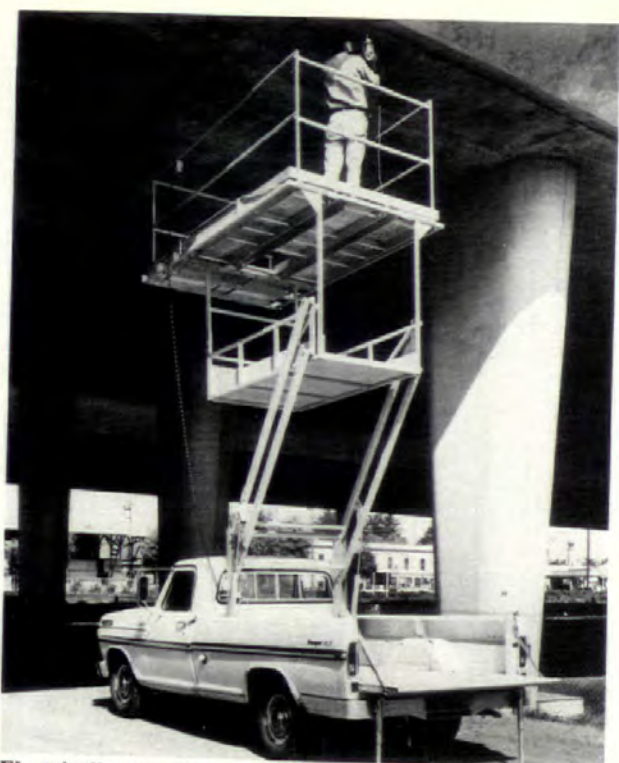
Electrically powered scaffold (above) has movable push-button controls. Unit with a 24' reach and a 1000-lb. capacity has a skidproof aluminum platform. Up-Mobile, Sacramento, CA. Circle 254 on reader service card.
