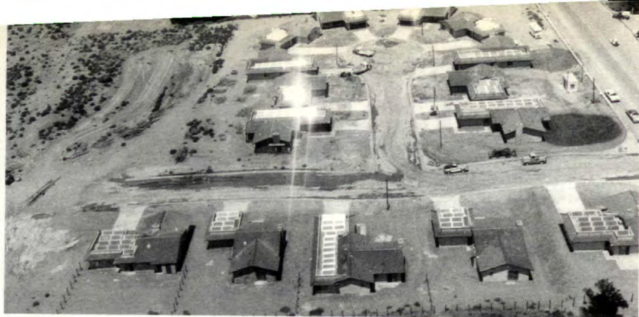
Solar-heated houses are sited in conventional subdivision fashion. Note that there are more solar collectors for the larger houses.
