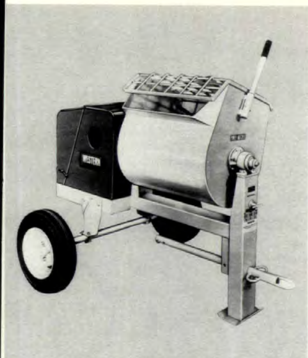
Mortar/plaster mixer (above) has a 5½ cu. ft. capacity. Unit features "two-in-one" blades—a regular steel blade for abrasive mixes is mounted over a full removable rubber blade that acts as a squeegee. Stow, Binghamton, NY. Circle 249 on reader service card
