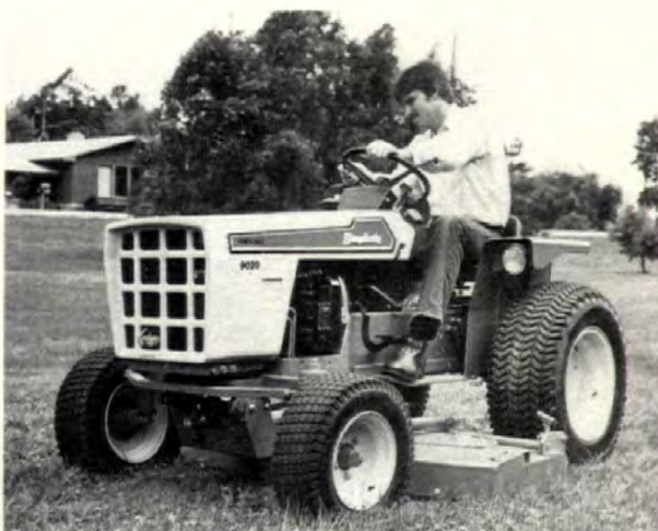
Garden tractor (above) features transmission shift interlock level which assures that the transmission remains in the selected range. A 48" tiller, 60" mower, 60" dozer blade and 60" grader blade are optional. Simplicity, Port Washington, WI. Circle 254 on reader service card
