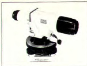
Automatic level (above) has front focusing for fast, smooth operation. Unit features three-point leveling with two screws and one pivot point. Keuffel & Esser, Morristown, NJ. Circle 250 on reader service card
