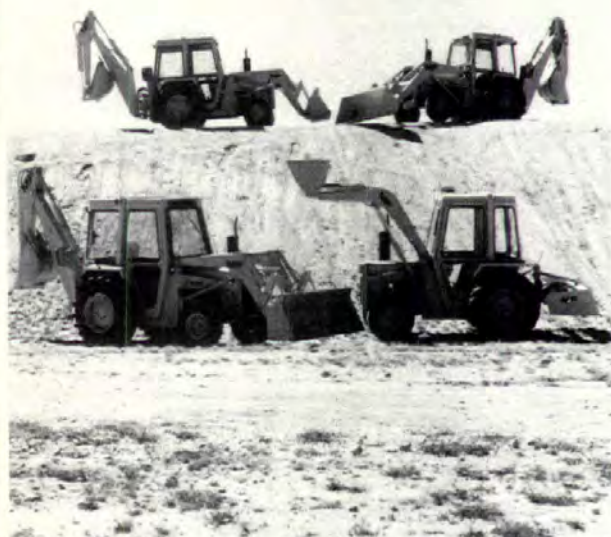
Tractor/backhoe/loaders (above) feature power steering with manual pump back-up. The units, with short turning radiuses, have breakout forces from 4500 lbs. to 8700 lbs. Massey-Ferguson, Des Moines, IA. Circle 248 on reader service card
