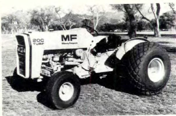
Turf tractor, "MF 20C" (above), features hydrostatic power steering and a heavy-duty, adjustable front axle. Unit has 8-speed transmission. Massey-Ferguson, Des Moines, IA. Circle 239 on reader service card
