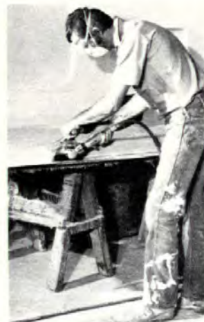
High-speed polisher (above) is a ½ hp unit that produces 1150 rpm. High-heat polishing hardens the shine to a mirror-like finish. American-Lincoln, Bowling Green, OH. Circle 244 on reader service card
