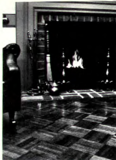
Hardwood flooring (above) features tongue-and-groove design. The 6"x6" squares come in six shades of wood and can be finished on the job. Flooring is installed without nails. The parquet flooring is suitable for commercial applications. Penn Wood, East Berlin, PA. Circle 216 on reader service card
