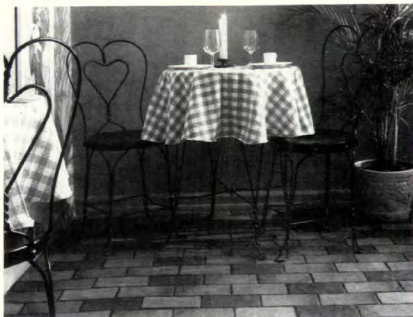
Unglazed ceramic tile, "Georgetown Blend" (above), is suitable for use on interior floors and walls, exterior walls not above the first floor level, vanity tops and countertops. The easy-to-install 8"x4" tiles may be arranged in a variety of patterns. The top and perimeter surfaces are irregular, creating a handcrafted effect. American Olean, Lansdale, PA. Circle 211 on reader service card
