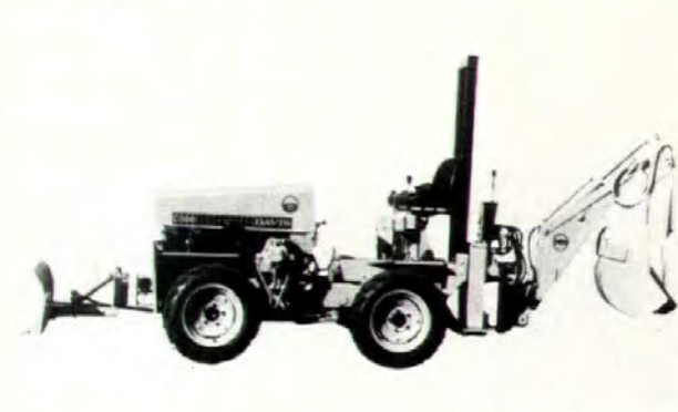
Backhoe and prime mover , "Fleethoe 30" (above), can be used for utility repairs and other operations where space is limited. The 56"-wide unit has an overall transport length of 178" with blade and backhoe attached. Davis Manufacturing, Wichita, KS. Circle 237 on reader service card
