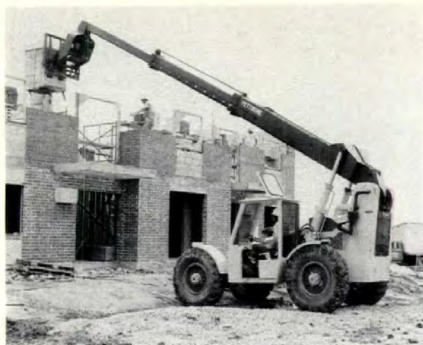
High-lift (above), with a hydraulically extending boom, is suitable for use on rough terrain. Unit has a maximum lifting capacity of 6,000 lbs. and a maximum working load of 2,150 lbs. The telescopic, self-leveling boom can reach out 20'10". Pettibone, Chicago. Circle 233 on reader service card
