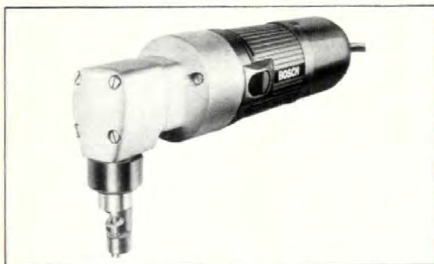
Sheet metal nibbler , "Model 1530" (above), is designed for tight curved as well as straight cuts. The lightweight tool makes random forms and internal cutouts from steel, aluminum and plastic up to .047" thick. Robert Bosch, Broadview, IL. Circle 234 on reader service card
