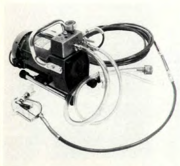
Portable airless electric paint sprayer , "ED-250" (above), is designed for small or short-run jobs. To reduce wear and conserve power, unit automatically shifts into neutral when the gun is closed. Device supports a spray tip up to .017". Graco, Minneapolis, MN. Circle 235 on reader service card
