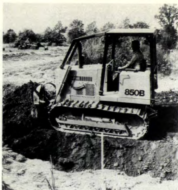
Crawler, "850B" (above), is designed for tight-quarter maneuvering, multi-job utilization and ease of transport. Unit has high torque capability at low engine-saving rpms. Attachment options include a 14' Case standard backhoe, integral arch design winch and parallelogram design five-shank ripper. The four-cylinder engine features direct injection fuel system. J.I. Case, Racine, WI. Circle 239 on reader service card
