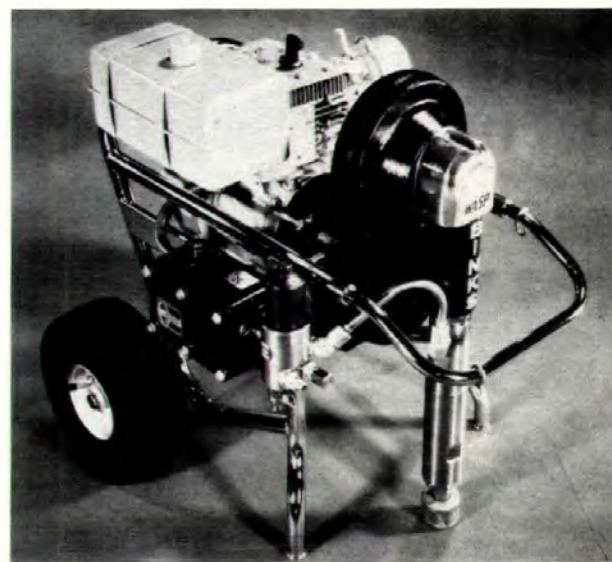
Gas-powered airless spraying unit , "Wasp" (above), operates for 3.5 hours on one gallon of gasoline. Portable unit delivers a gallon per minute at up to 3,000 psi pressure. Device can spray a range of materials including stains and lacquers. Binks, Franklin Park, IL. Circle 238 on reader service card
