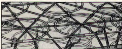
Eight-way hand-tied springs are found in the finest upholstered pieces.
