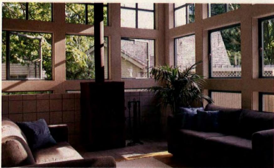
To make the most of Seattle's damp, gray climate, the maximum legal window area is used together with a tiled concrete wall that retains heat.
