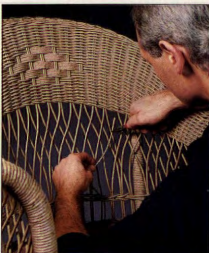
8. Replace spokes by pushing them into place with needle-nose pliers, following the pattern of the weave.
