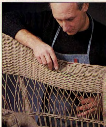
6. Weave in the new wicker, starting from the underside. Follow the weave's pattern, pulling wicker tight as you go.
