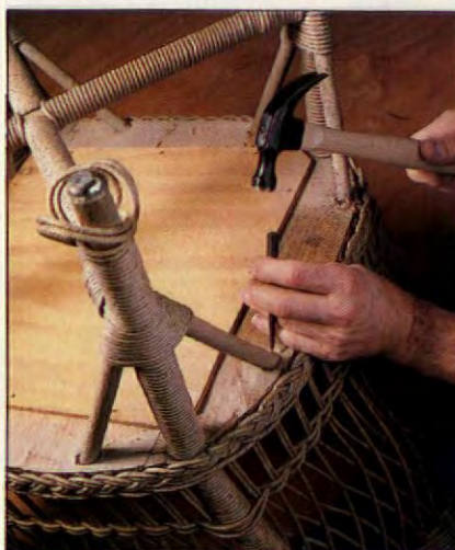
2. Glue and renail any loose parts of the understructure; set nailheads. Tighten or replace any missing screws.
