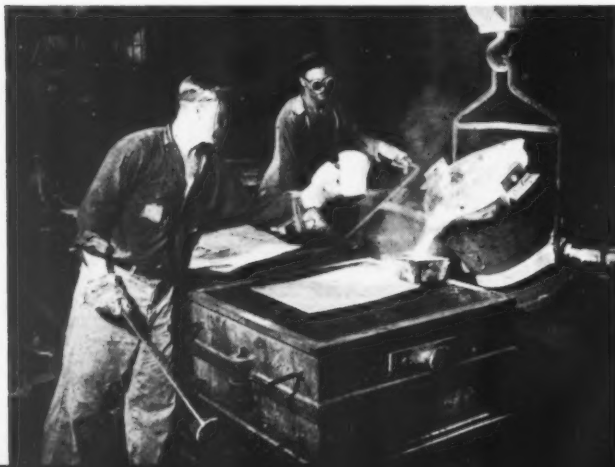
MOLTEN MAGNESIUM BEING POURED FROM CRUCIBLE INTO A SAND MOLD. SHAKING INHIBITORS ON METAL PREVENTS BURNING.
