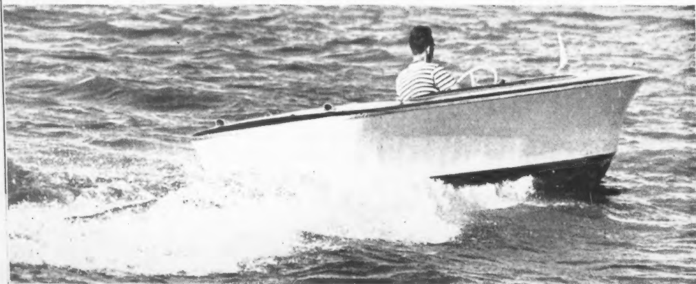
The "Gar-Form" to be manufactured in quantity of low-pressure molded fiberglass and plastic.
