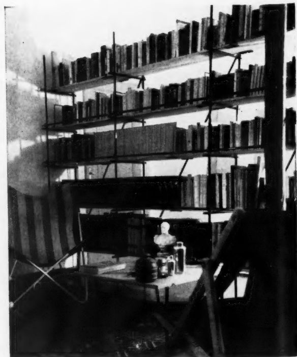
The steel and aluminum scaffolding which holds a book load of 500 pounds, screens the entrance door.
