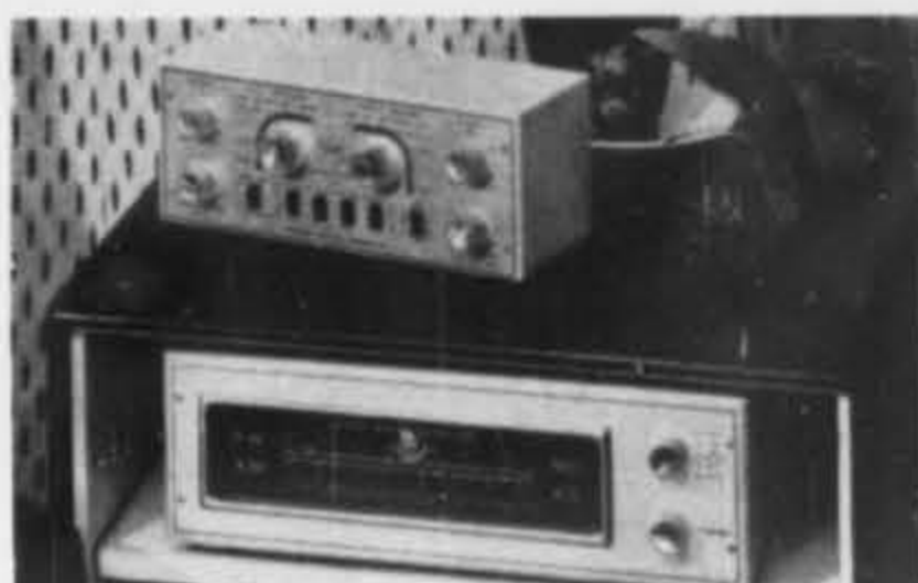
Newcomb Audio Products' "Compact" AM-FM tuner (in shelf) and "Classic" 2500R amplifier-preamplifier (on top), both in satin-gold cabinets. The tuner has an output jack to permit adaptation for binaural. FM frequency response from 20 to 20,000 cycles. Preamp allows 36 recording curves.
