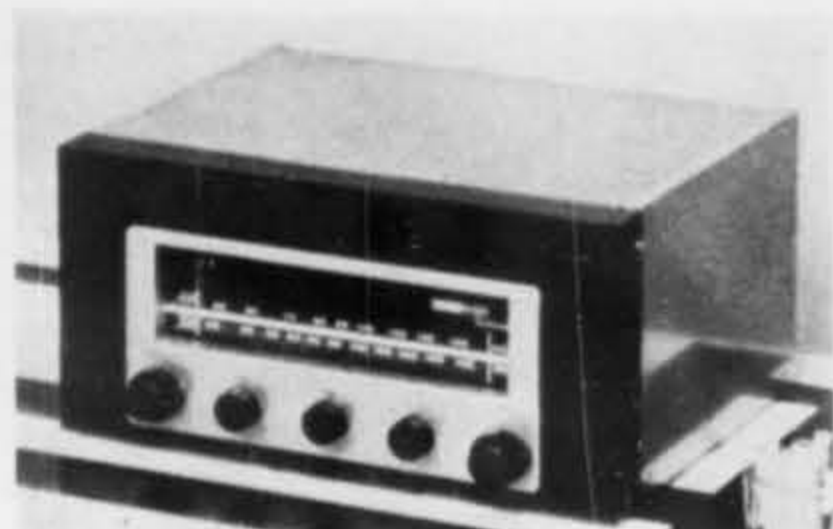
Harman-Kardon "Festival" D-1100 combines an AM-FM tuner, a preamplifier, and a 30-watt power amplifier. Five control knobs: (1) Volume and "Contour," the latter to retain bass and treble at low volume; (2) Bass; (3) Function—AM, FM, Auxiliary, three record curves; (4) Treble; (5) Tuning.
